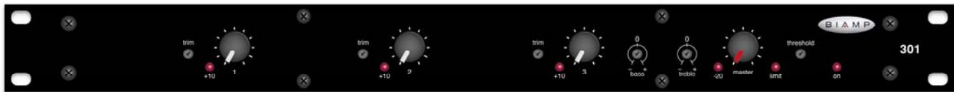
**Trim:** These screwdriver adjustable controls provide 40dB of gain adjustment to compensate for different input signal levels. For best performance, adjust Trim so the +10 Indicator flashes only on occasional peaks in signal level (see +10 Indicator below).
