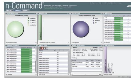
The ADTRAN n-Command MSP GUI enables the network administrator to quickly and easily organize all the managed devices. To promote flexibility and customization for each n-Command MSP user, the system is designed so each user can drag and drop modules and resize or move them around within the screen to tailor the views.
