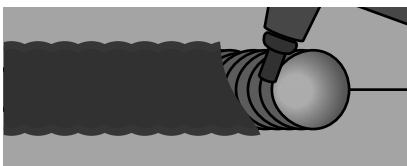
PARTIALLY CHIPPED AWAY TO SHOW WELD
