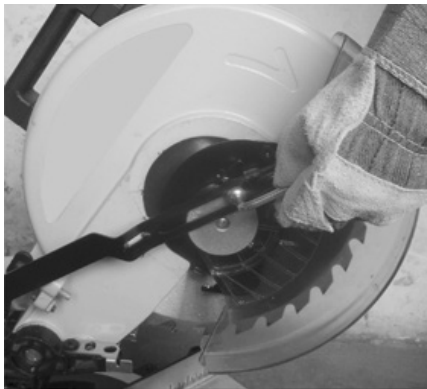
Figure D: Removing Safety Screw
