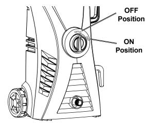
**NOTICE:** Pressure Washer will run **only** while Trigger is pressed. When trigger is released, Pump will turn off. **Do not leave idle for more than one minute without spraying.**
