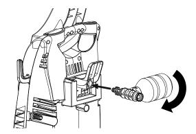
Store in a dry, frost-free room. Flush the unit with automotive antifreeze prior to long-term storage.
