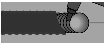
PARTIALLY CHIPPED AWAY TO SHOW WELD
