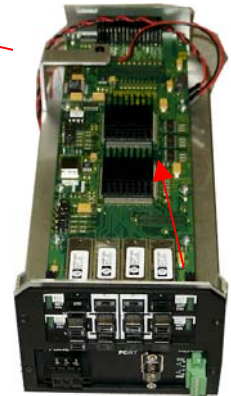
Figure 3.6.2f: Securely latching up 6KPMV Cards into a Magnum 6K8-Series Step 6. Now screw
