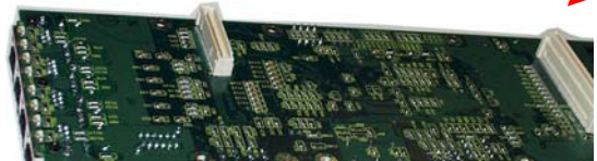
Fig 3.6.2e Daughter Board shown upside down with two male latch connectors
