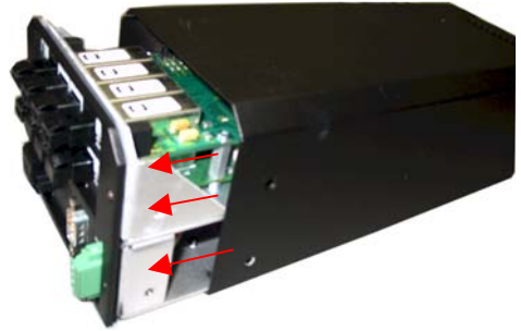
Figure 3.6.1a: Removing the Top panel from the Chassis base of the unit
