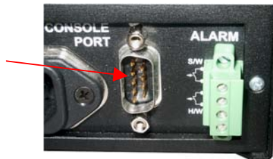
Fig 3.7 Enlarged view of Magnum 6K8-Series Console Port area
