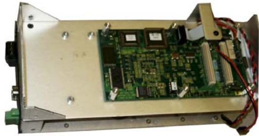
Fig 3.6.2a A Magnum 6K8 unit with main board (motherboard) only
