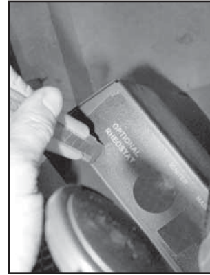
Figure 8.21 Cut out the rheostat/speed control cover on rear shield. Re-install rear shield.
