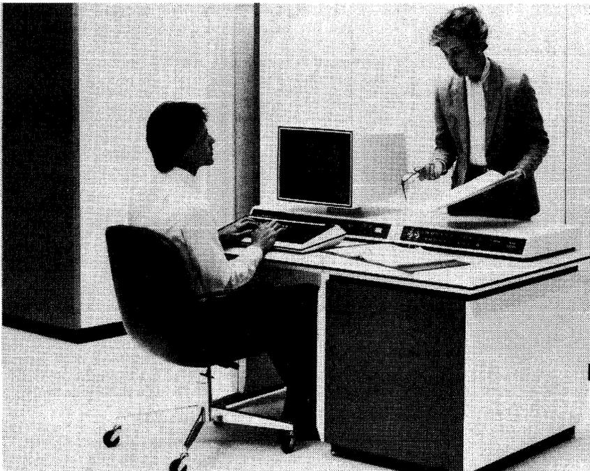
*The Amdahl Model 5860 is the most powerful uniprocessor that Amdahl has ever produced. This member of the Amdahl 580 family represents an evolutionary extension to the product line and offers a compatible growth path for Amdahl 470 users. The 5860 has twice the processing power of Amdahl's 470V/8. Standard features on the 5860 include 16 I/O channels, 16MB of main storage, two 32K high-speed buffers, power distribution unit, system console and air cooling.*
