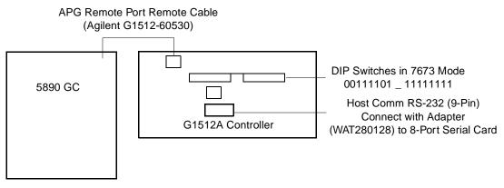
Figure 2-6 Connecting a 5890 GC and G1512A Controller
