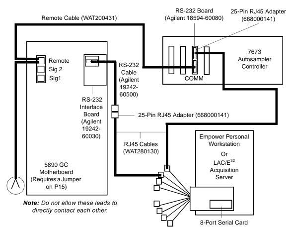
Figure 2-2 Connecting a 5890 GC and 7673 Controller to the Serial Card
