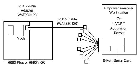
Figure 2-4 Connecting a 6890 Plus GC or 6890N GC to the Serial Card
