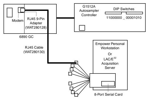
Figure 2-3 Connecting a 6890 GC and G1512A Controller to the Serial Card
