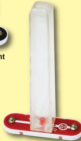
Light Tower LED attachment mounted to D1
