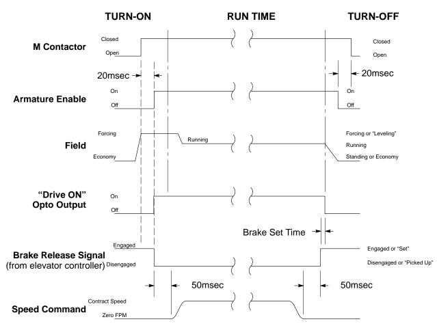
Figure 5-4 Typical Power Up/Down Sequence for DC SCR Controls.
