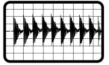
Relay and Contactor Coils Among the most common sources of noise are the ever–present coils of contactors and relays. When these highly inductive coil circuits are opened, transient conditions often generate spikes of several hundred volts in the control circuit. These spikes can induce several volts of noise in an adjacent wire that runs parallel to a control–circuit wire.
