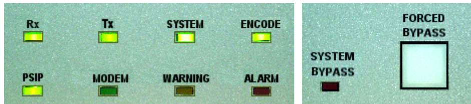
Figure 8: Front Panel LED Indicators
