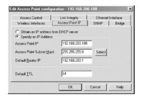
One nice thing about the AP Manager is that assigning the subnet mask is especially easy. The Select button raises a subnet mask panel that shows the mask in dotted decimal, hexadecimal, and mask-length notations. See Figure 14-3.
