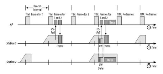
Figure 7-11. Buffered frame retrieval process
