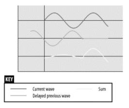
With OFDM, inter-symbol interference does not pose the same kind of problem. The Fourier transform used by OFDM distills the received waveform into the strengths of the subcarriers, so time shifts do not cause dramatic problems. In <u>Figure 11-4</u>, there would be a strong peak for the fundamental low-frequency carrier, and the late-arriving high-frequency component could be ignored.
