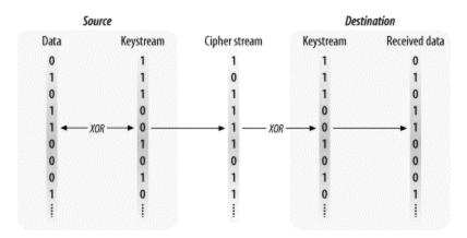
Most stream ciphers operate by taking a relatively short secret key and expanding it into a pseudorandom keystream the same length as the message. This process is illustrated in Figure 5-2. The pseudorandom number generator (PRNG) is a set of rules used to expand the key into a keystream. To recover the data, both sides must share the same secret key and use the same algorithm to expand the key into a pseudorandom sequence.
