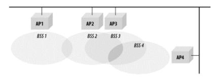
Figure 2-7. Overlapping BSSs in an ESS
