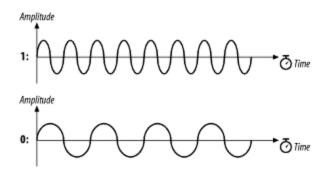
The rate at which data is sent through the system is called the *symbol rate*. Because it takes several cycles to determine the frequency of the underlying carrier and whether 1 or 0 was transmitted, the symbol rate is a very small fraction of the carrier frequency. Although the carrier frequency is roughly 2.4 GHz, the symbol rate is only 1 or 2 million symbols per second.
