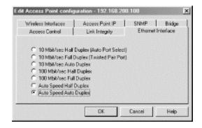
Figure 14-6. Ethernet interface configuration
