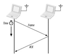
The sequence in <u>Figure 3-1</u> is an *atomic* operation. 802.11 allows stations to lock out contention during atomic operations so that atomic sequences are not interrupted by other stations attempting to use the transmission medium.
