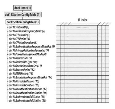
All entries in the station configuration table start with the prefix dot11smt.dot11StationConfigTable.dot11StationConfigEntry (1.1.1):
