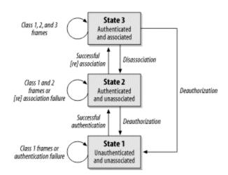
Figure 4-48. Overall 802.11 state diagram
