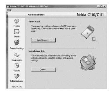
To access the smart-card functions, click on the **Add/Remove...** button at the top of the page. This brings you to <u>Figure 12-23</u>, which allows you to erase the smart card and move profiles from disk to smart card and vice versa.
