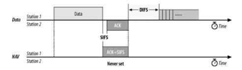
The frame uses the NAV to reserve the medium for the frame, its acknowledgment, and the intervening SIFS. By setting a long NAV, the sender locks the virtual carrier for the entire sequence, guaranteeing that the recipient of the frame can send the acknowledgment. Because the sequence concludes with the ACK, no further virtual carrier locking is necessary, and the NAV in the ACK is set to 0.
