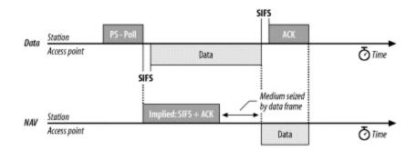
If the buffered frame is large, it may require fragmentation. <u>Figure 3-20</u> illustrates an immediate PS-Poll response requiring fragmentation. Like all other stations, access points typically have a configurable fragmentation threshold.
