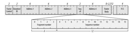
Higher-level frames are each given a sequence number as they are passed to the MAC for transmission. The sequence number subfield operates as a modulo-4096 counter of the frames transmitted. It begins at 0 and increments by 1 for each higher-level packet handled by the MAC. If higher-level packets are fragmented, all fragments will have the same sequence number. When frames are retransmitted, the sequence number is not changed.
