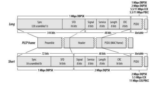
Naturally, the optional short format may be used only if all stations support it. To prevent networks configured for the short format from disappearing, 802.11b requires that stations answering Probe Requests from an active scan return a response using the same PLCP header that was received. If a station that supports only the long PLCP header sends a Probe Response, an access point returns a response using the long header, even if the BSS is configured for the short header.
