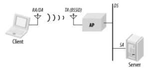
Frames are created by the server, so the server's MAC address is the source address for frames. When frames are relayed through the access point, the access point uses its wireless interface as the transmitter address. As in the previous case, the access point's interface address is also the BSSID. Frames are ultimately sent to the client, which is both the destination and receiver.
