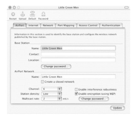
Figure B-12. Wireless interface configuration
