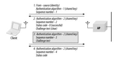
Figure 7-5. Shared-key authentication exchange
