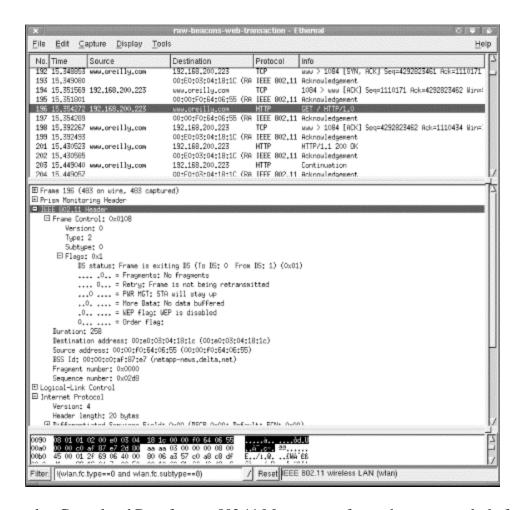
Compared to Control and Data frames, 802.11 Management frames have a great deal of structure. Ethereal decodes Management frames into two parts. *Fixed Parameters* in the tree view pane correspond to the fixed fields of 802.11 management frames. *Tagged Parameters* are the variable fields and are decoded in the tree view pane. <u>Table 16-2</u> shows the fixed fields that can be searched on in Ethereal, as well as the capability flags.
