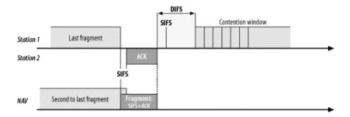
4. If the More Fragments bit in the Frame Control field is set to 1, more fragments remain. The Duration field is set to the amount of time required for transmission of two acknowledgments, plus three short interframe spaces, plus the time required for the next fragment. In essence, nonfinal fragments set the NAV just like an RTS would (Figure 4-3); for this reason, they are referred to as a *virtual RTS*.
