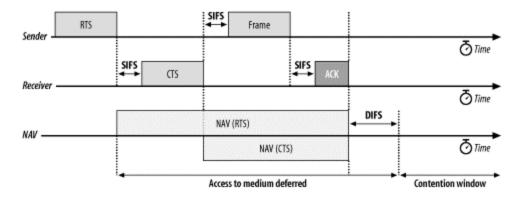
Figure 3-5. Using the NAV for virtual carrier sensing
