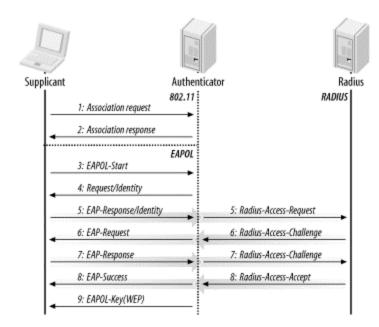
Figure 6-9. EAPOL exchange on an 802.11 network
