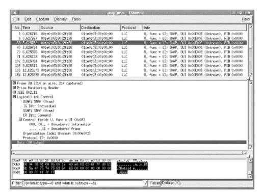
The data is encapsulated in a raw LLC frame using the Unnumbered Information header. The OUI used is assigned to Nokia Wireless Business Communications, the wireless LAN product unit of Nokia. (The listing of assigned OUIs can be found at <a href="http://standards.ieee.org/regauth/oui/oui.txt">http://standards.ieee.org/regauth/oui/oui.txt</a>.) In the LLC data, the name of the access point, Outside, is plainly clear.
