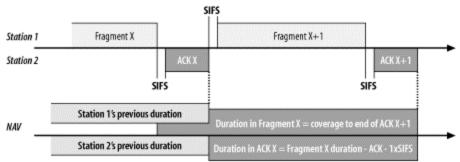
Figure 4-18. Duration in non-final ACK frames
