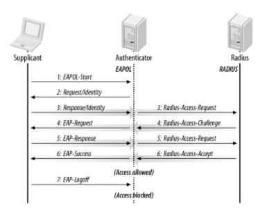
Figure 6-8. Typical EAPOL exchange
