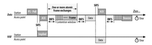
After receiving a data frame, the station must remain awake until the next Beacon is transmitted. Beacon frames only note whether frames are buffered for a station and have no way of indicating the number of frames. Once the station receives a Beacon frame indicating that no more traffic is buffered, it can conclude that it has received the last buffered frame and return to a low-power mode.
