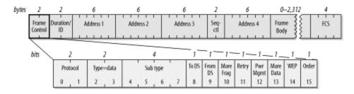
In <u>Table 3-1</u>, bit strings are written most-significant bit first, which is the reverse of the order used in <u>Figure 3-10</u>. Therefore, the frame type is the third bit in the frame control field followed by the second bit (b3 b2), and the subtype is the seventh bit, followed by the sixth, fifth, and fourth bits (b7 b6 b5 b4).
