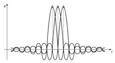
OFDM takes the coded signal for each subchannel and uses the inverse fast Fourier transform (IFFT) to create a composite waveform from the strength of each subchannel. OFDM receivers can then apply the FFT to a received waveform to extract the amplitude of each component subcarrier.
