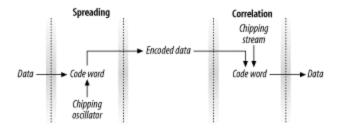
Barker spreading, as used in the lower-rate, direct-sequence layers, uses a static code to spread the signal over the available frequency band. CCK uses the code word to carry information, as well as simply to spread the signal. Several phase angles are used to prepare a complex code word of eight bits.
