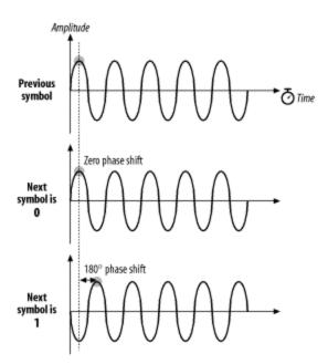
Figure 10-19. DBPSK encoding
