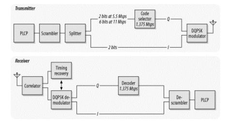
Figure 10-28. HR/DSSS transceiver
