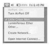
In <u>Figure B-4</u>, there are two networks within range: Little Green Men and Luminiferous Ether. The checkmark by Little Green Men indicates that it is the network to which the user is currently connected, though the user can switch between the two networks simply by selecting a preference. Any other network can be selected by using the Other... option and entering the name of the network.
