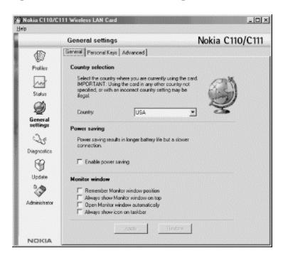
By default, the driver manages TCP/IP properties and other network configuration and treats 802.11 network names as case-sensitive network identifiers. All of these can be changed by using the General settings  $\rightarrow$  Advanced tab (Figure 12-14).
