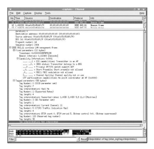
At the end of the Beacon is a variable field with a reserved tag number that the wireless card's vendor uses to hold the access point's name, and possibly the access point's load factor. The ASCII dump displays the word Outside clearly, which is, in fact, the name of this access point.
