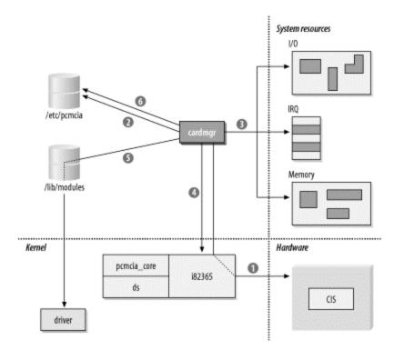
Figure 13-1. Linux PCMCIA configuration system
