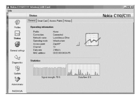
When troubleshooting connectivity problems or expanding a network, it can be useful to run a card as a scanner, simply to see the access points within range. For example, you can walk around a building with your laptop and ensure that at least two access points are reachable in high-traffic areas. Like the general statistics page, the access point listing is reached as a tab off the status page.
