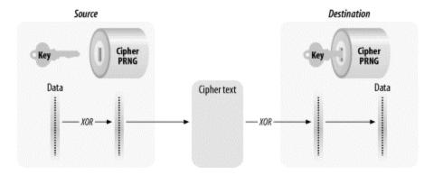
Because the security of a stream cipher rests entirely on the randomness of the keystream, the design of the key-to-keystream expansion is of the utmost importance. When RC4 was selected by the 802.11 working group, it appeared to be quite secure. But once RC4 was selected as the ciphering engine of WEP, it spurred research that ultimately found an exploitable flaw in the RC4 cipher that will be discussed later.
