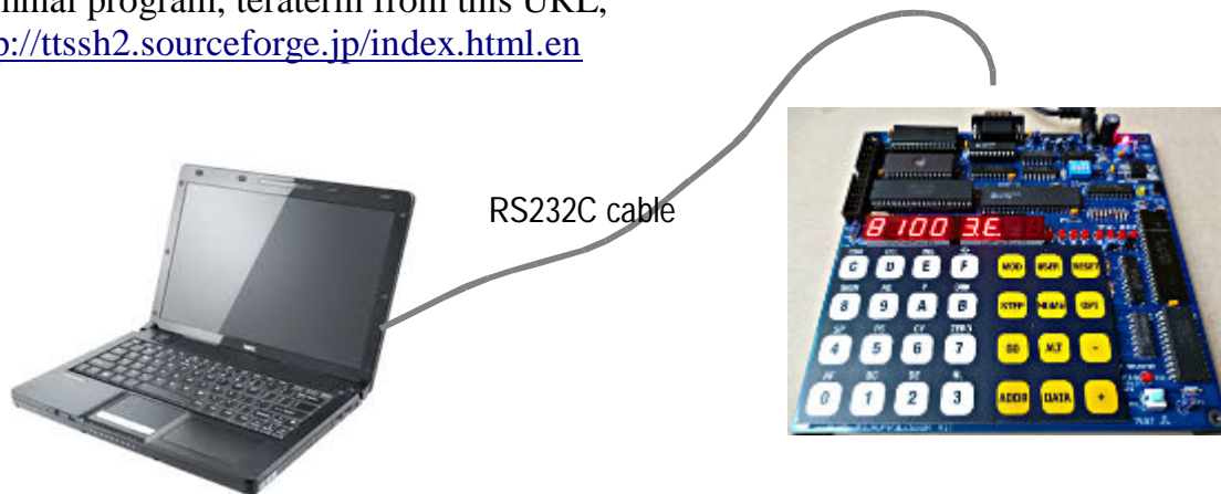
Figure 7: Connecting PC running teraterm and kit with RS232 cross cable.
