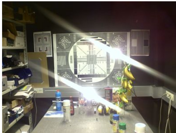
Figure 29 Image of point light sources taken with a dirty (finger print) protective window
