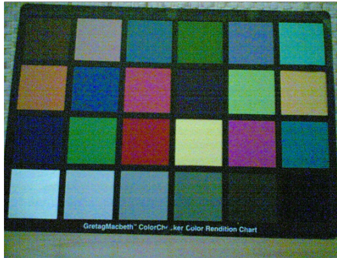
Figure 19 Noisy image taken in +70 degrees Celsius
