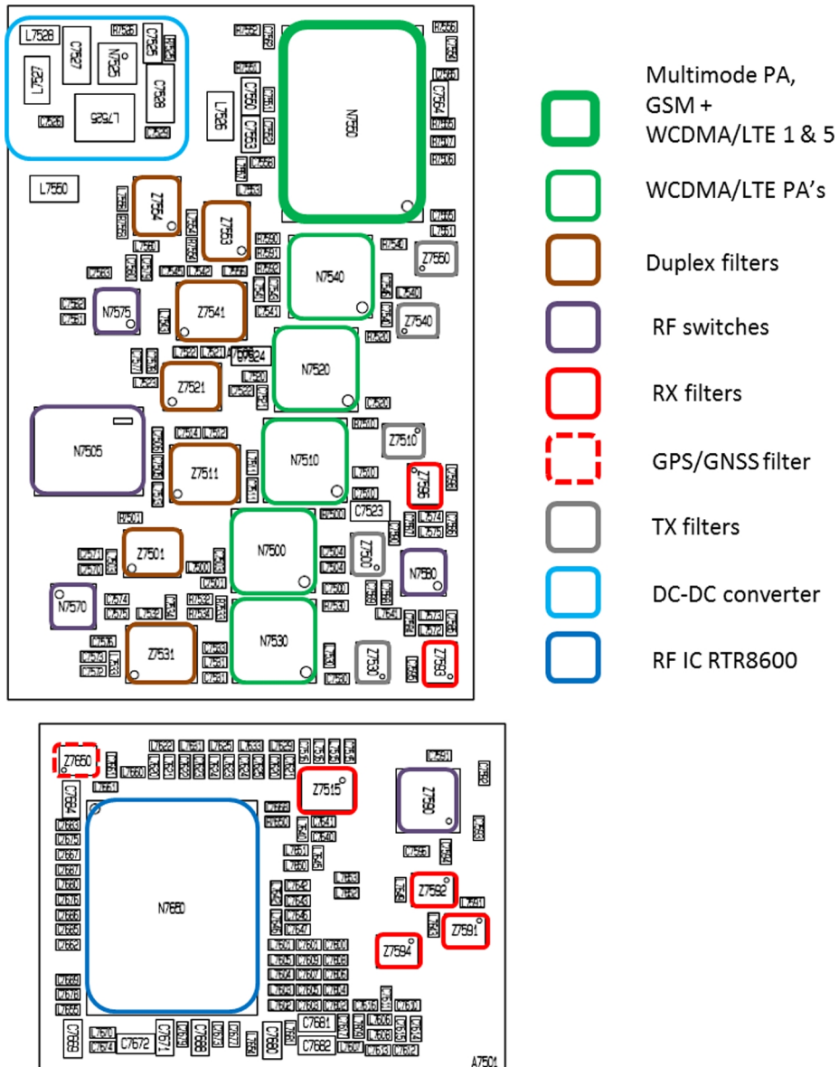
Figure 11 RF key components
