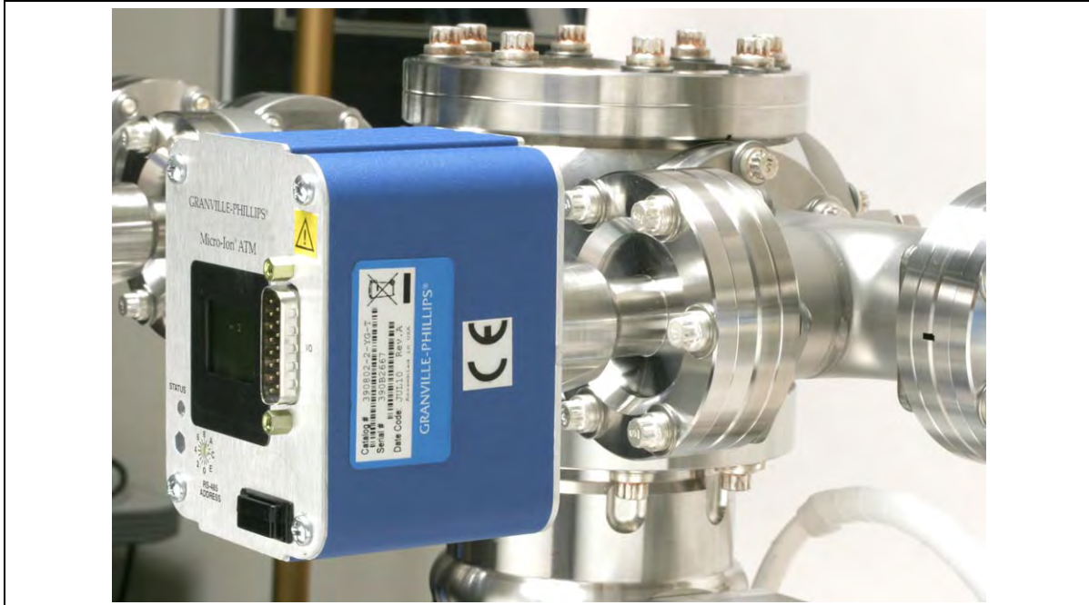
Figure 3-6 Micro-Ion Gauge Mounted on a Vacuum Chamber
