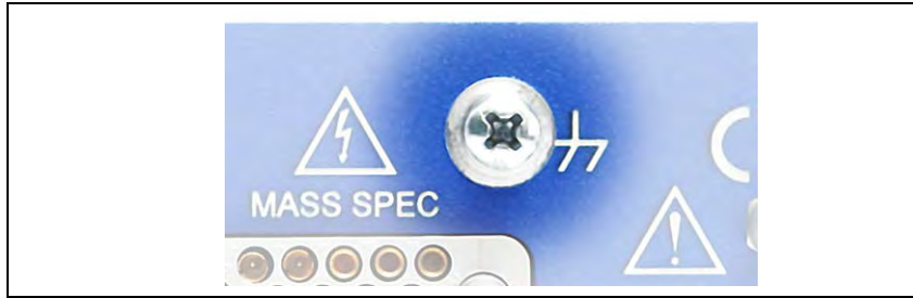
Figure 5-6 Ground Connection on the Rear of the VQM Controller
