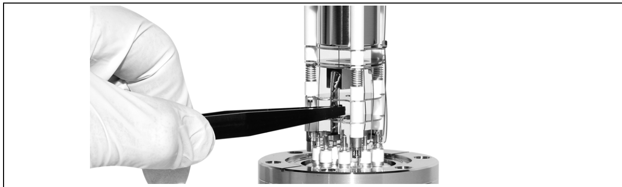
Figure 7-11 Remove the Electron Multiplier
