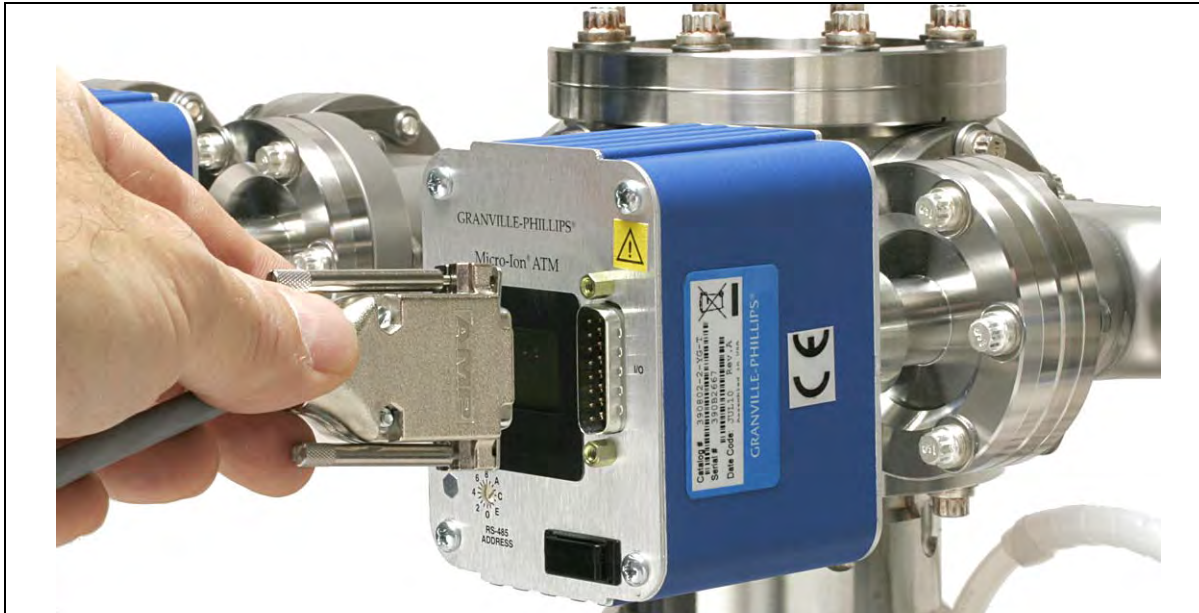
Figure 3-12 Connect the Cable to the Micro-Ion Gauge
