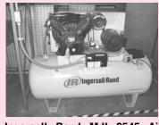
Ingersoll Rand Mdl 2545 Air Compressor; 175 PSIG, 2 Cyl w/120 Gal Horz Tank
