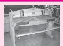
Pexto Mdl 152-K Sheet Metal Shear; 52", Cap, 16 Gauge Soft Steel w/Back Gauge
