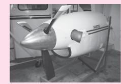
Avotek Mdl E-47 Turbine Eng Removal & **Replacement System Trainer for PT-6** Engine
