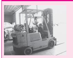
Mitsubishi Mdl FGC25 Fork Lift; 4000 lbs Hard Rubber Tires, 3 Stage, 18' Mast, Side Shifting Forks, Propane
