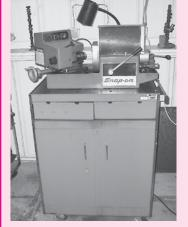
Snap-On/Kwik Way Mdl SVS Wet Valve Facer w/Rocker Arm Attachment (Near New)
