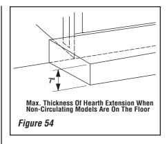
Secure the hearth extension to the floor to prevent possible shifting.
