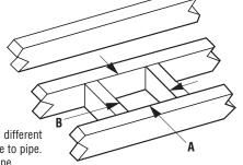
**Note:** Faming Dimensions in Canada & USA are different because installations in USA require 1" Clearance to pipe. Installations in Canada require 2" Clearance to pipe.
