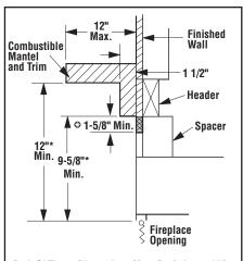
\*Both Of These Dimensions Must Be At Least 18" When An Unvented Gas Log Set Rated At 26,000 BTU Or Higher Is Used. (Maximum 40,000 BTU).
