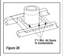
Security's chimney sections do not need to be screwed together. Additional reinforcement is not necessary except in certain offset conditions (refer to *Page 16, Figure 47*).
