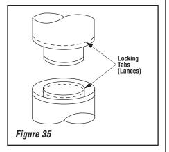
**Note:** Assemble one component of chimney at a time (inner section first, then outer section last) before proceeding with the next complete section.
