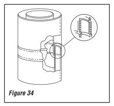
The outer chimney section installs the oppositeway; the lanced end goes down and each new section goes OVER the outside of the previous section installed (*Figure 35*).
