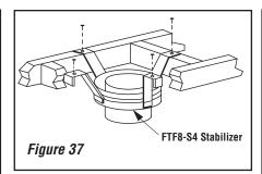
**Note:** Do not apply excessive pressure to any subsequent chimney sections following the stabilizer when installing. Ensure each subsequent chimney section is securely attached by testing as noted in **Step 4**.
