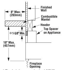
© The shaded gray area showing 1-5/8" Min. indicates non-combustible materal is required.
