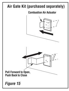
To operate, push the end of the actuator arm to the left as shown in *Figure 15*, until it "pops" free of its "locked" position. Pull the actuator forward to open the combustion air door, and push it back to close. To "lock" the combustion air door closed, ensure the actuator is pushed all the way back then push the end of the actuators to the right until the step in the actuator moves behind the appliance front face within the slotted opening.
