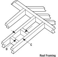
**Note:** Faming Dimensions in Canada & USA are different because installations in USA require 1" Clearance to pipe. Installations in Canada require 2" Clearance to pipe.
