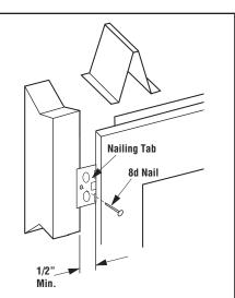
**Note:** The nailing tab and the area directly behind the nailing tab is exempt from the clearances described on **Page 5**. Maintain at least 1/2" clearance from the firebox wrapper to the framing at the closest point of contact, directly adjacent to the flange.
