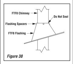
**Note:** Do not caulk or seal the ventilating openings or seal the flashing at the chimney.
