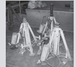
(3) Columbus Tripod Aircraft Jacks, 10 Ton, 38"
