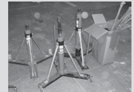
Alpha Low Wing Jacks w/Extensions, Mdl 838, 8 Ton
