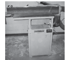
Powermatic Belt Sander, Mdl 13, 6"x40" w/1 1/2 HP Motor Dremel 16" Variable Speed Scroll Saw, Mdl 1680
