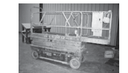
Genie Elect Scissor Lift, Mdl GS-2032, Max Platform Height 20' w/Extending Platform, 800 Lb Cap
