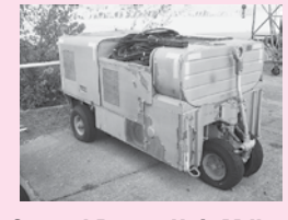
Ground Power Unit Mdl MD3A w/6 Cyl Packet
