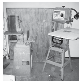
Rockwell Belt/Disc Sander, Mdl 31-71, 6" Belt, 12" Disc
