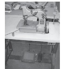
KARPET King HD Commercial Surging Machine Mdl 812K w/Table
