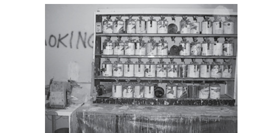
Dedco 48 Can Digital Paint Storage/Mixing System, Mdl RJ 88 Franklin Shadowgraph Triple Beam Mixing Scale Fairbanks Digital Platform Scale, Mdl HR-5000-1 Red Devil Dual 1 Gal. Paint Shaker (3) Binks 3 Gal Paint Pots Cobalt Gravity Flow Paint Gun Grayco Pneumatic 55 Gal Barrel Pump
