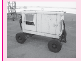
Hobart Jet Ex-2 GPU, 28 Volt, 700-1300 Amp, 21 KW w/Ford 6cyl Industrial Eng
