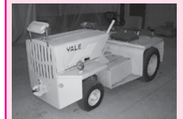
Yale Mdl G10P40-CF Tug 4000 Lb DBP, 4 Spd Manual w/Gas Flat Head 6 Cyl Eng
