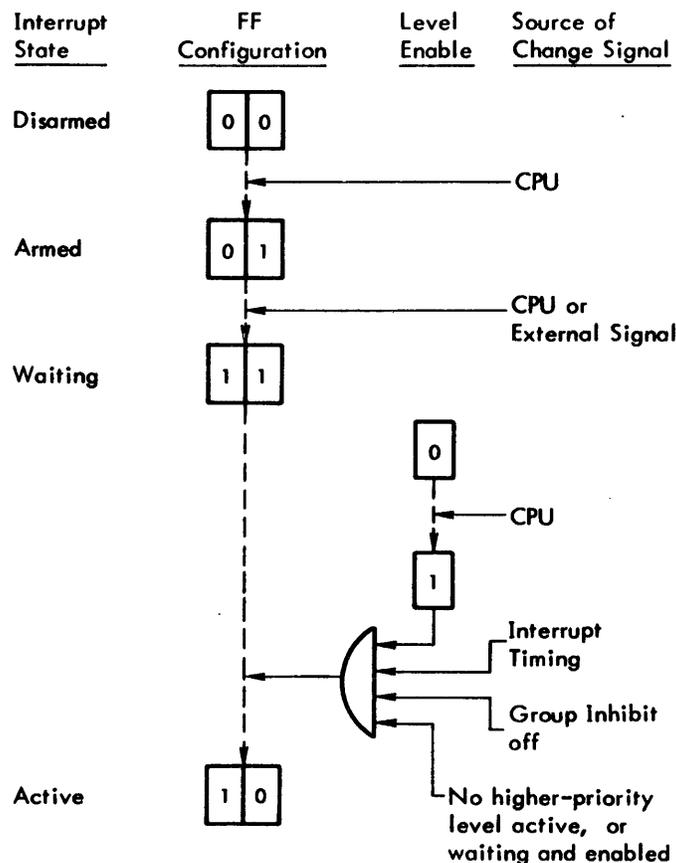
Figure 7. Interrupt Level Operation
