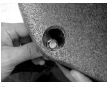
This picture shows the enclosure from the bottom after both holes have been drilled. The bolt is shown in its eventual location.
