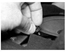
**STEP 3:** Remove the rear factory speakers.
