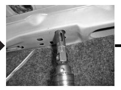
**STEP 10:** This is a picture from the passenger side trunk area. Drill the 3/4" hole behind of pre-existing square hole.
