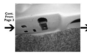
**STEP II:** Insert the supplied u-bolt into the hole drilled in Step 10. The threaded portion of the u-bolt should be aligned with the preexisting square hole located directly beneath the newly created round hole. This threaded section will receive a 1/4" bolt used to secure the enclosure.
