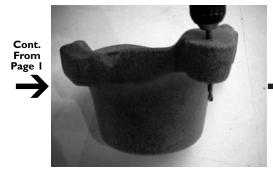
**STEP 7:** Using a 1/4" drill bit, drill out the correct holes. Make sure to go through both layers of the enclosure. The drill bit must be kept straight while drilling.
