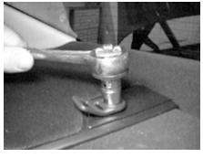
**STEP 1:** Remove the plastic housing and bolt from the bracket located on the rear speaker grills.
