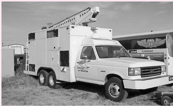
1988 Ford F-350 Custom De-Ice Truck, V8 Gas, Auto Trans., Superior Mdl M5000 De-Ice System, Telsta Boom System Mdl A28DEM, 28' Platform Height, Single Boom Nozzle, Isuzu 3-Cyl Diesel Generator, 3-Burner Heater
