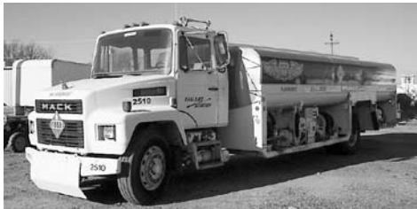
1991 Mack Jet A Fuel Truck, Diesel Engine, Auto Trans., 5,100 Gal Stainless Steel Tank, Single Pump & Meter w/Dual Front Reels, Single Point & Over Wing Nozzles, Priest Injectors, Single Pump & Reel w/Over Wing Nozzle at Rear, Bottom & Top Load, Fuel & De-Fuel Capable, 300 Gal/Minute Flow Rate Filters
