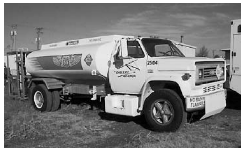
1987 Chevy 70 Avgas Truck, 8 Cyl Gas, 4-Speed Trans., 2,200 Gal Stainless Tank, Top & Bottom Load, Fuel/De-Fuel Capable, Dual Pumps, Meters & Reels, Dual Over Wing Nozzles, All Rear Mounted
