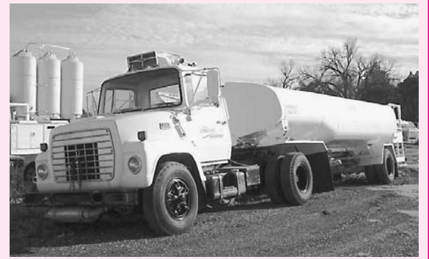
1979 Ford 7000 Tractor Tanker Truck, Cat 3208 Diesel, 5-Speed Trans., 5,000 Gal Steel Glycol Tank, Top & Bottom Load, Dual Reels, Faucet Filter System, Single Meter
