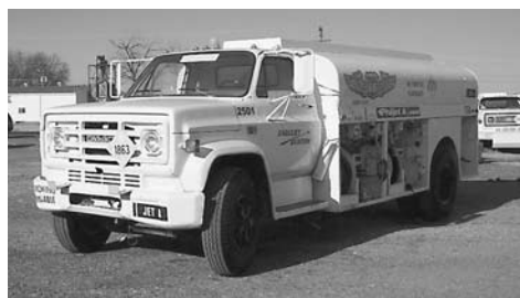
1980 GMC 7000 Jet A Fuel Truck, V-8 Gas, 5-Speed Trans, 2,500 Gal Steel Coated Tank, Dual Pumps, Meters & Reels, Over Wing & Single Point Nozzles, Fuel/De-Fuel Capable, Top & Bottom Load
