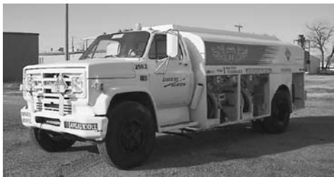
1980 GMC 7000 Avgas Truck, V-8 Gas Engine, 5-Speed Manual Trans., 2,500 Gal Steel Coated Tank, Bottom & Top Load, Dual Meters, Pumps & Reels, Dual Over Wing Nozzles
