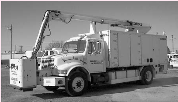
1998 Navistar International 4700 De-Ice Truck, Diesel Engine, Auto Trans., Has Global Mdl 2100BLNR De-Ice Unit, 1,900 Gal Type 1 & 200 Gal Type 4 Tanks, 47' Boom Platform Height, 3,000 PSI Operating Pressure, Dual Boom Nozzles, 4-Burner Heater, Single Nozzle Rear Reel
