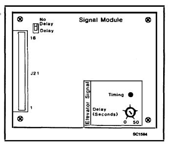
**FIGURE 6-5. SIGNAL MODULE**
