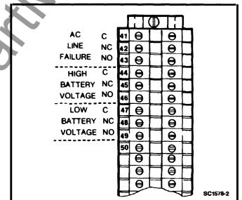
FIGURE 5-11. 10-AMP CHARGER ALARM CONTACTS
