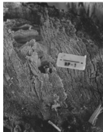
Figure 2—Signumat tag in a log.
