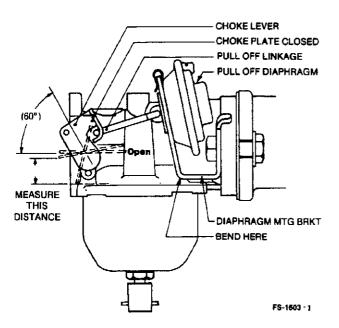
FIGURE 6-25. CHOKE PULL-OFF DIAPHRAGM
