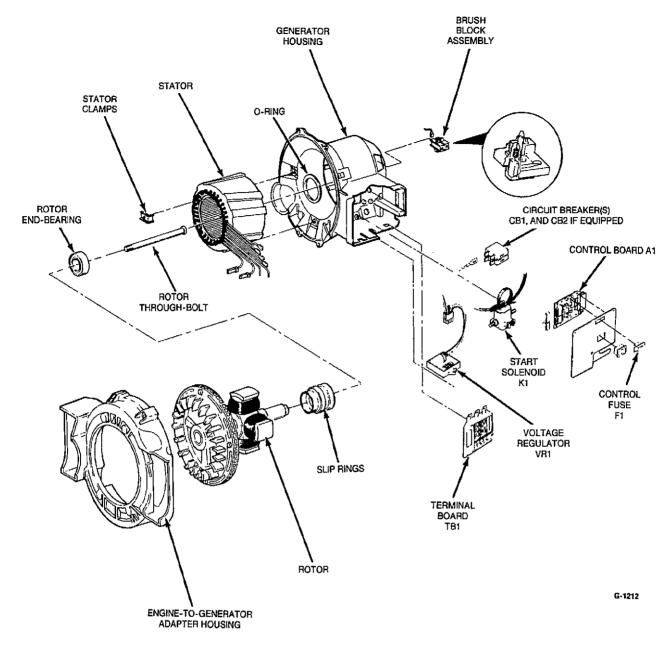
FIGURE 8-1. GENERATOR CONTROL COMPONENTS
