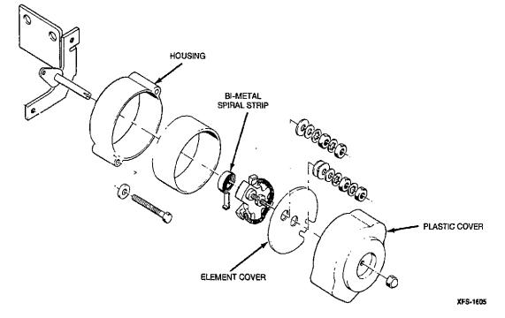
FIGURE 6-23. CHOKE ASSEMBLY
