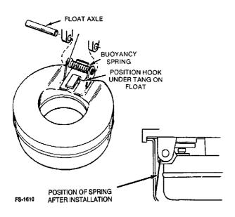
FIGURE 6-21. FLOAT INSTALLATION
