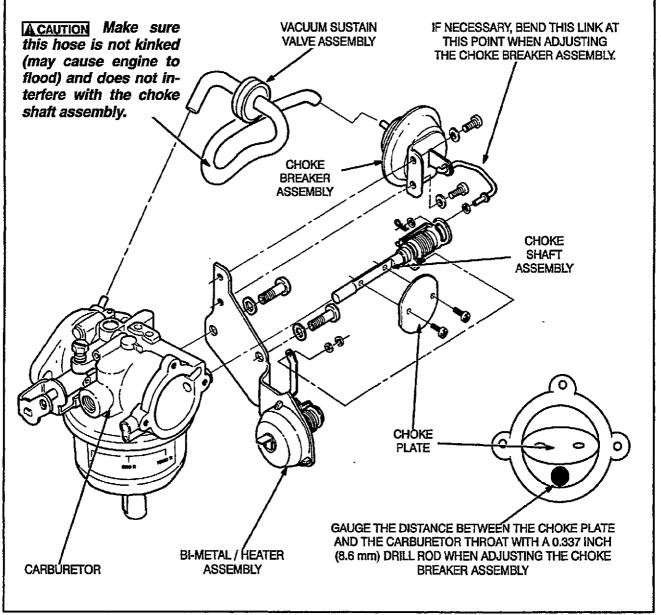
FIGURE S-5. CHOKE ASSEMBLY
