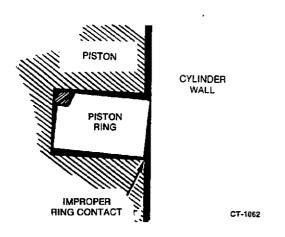
FIGURE 9-22. NEW RING IN WORN RING GROOVE
