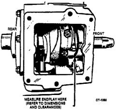
FIGURE 9-28. CHECKING ENDPLAY
