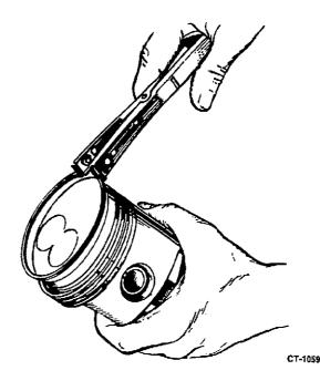
FIGURE 9-19. REMOVING PISTON RINGS
