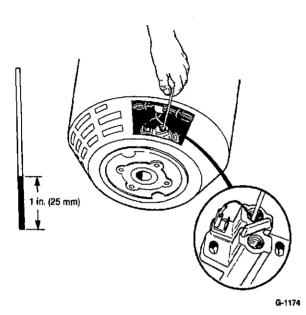
FIGURE 8-11. CHECKING BRUSH WEAR
