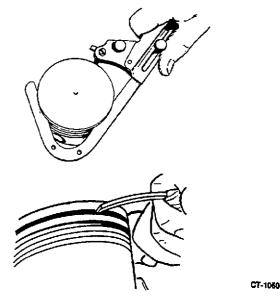
FIGURE 9-20. CLEANING RING GROOVES
