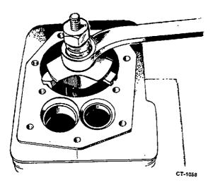
FIGURE 9-18. REMOVING WEAR RIDGE
