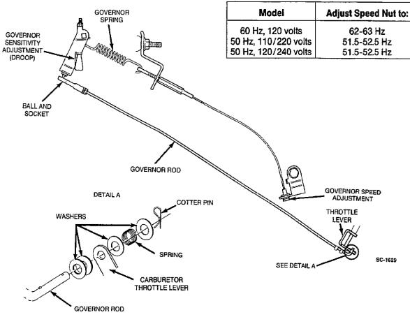
FIGURE 6-14. GOVERNOR ADJUSTMENT (SPEC H)
