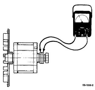
FIGURE 8-15. TESTING ROTOR FOR OPENS OR SHORTS
