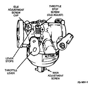
FIGURE 6-18. CARBURETOR FUEL ADJUSTMENTS
