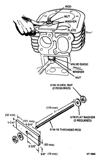
FIGURE 9-9. VALVE GUIDE INSTALLATION
