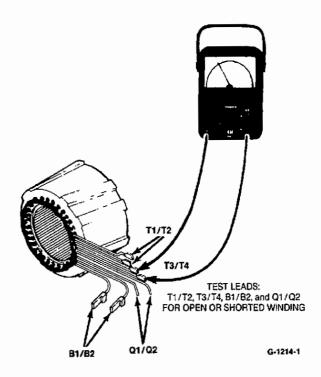
FIGURE 8-17. TESTING STATOR FOR OPENS OR SHORTS
