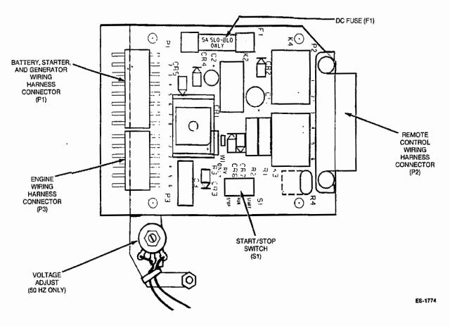
FIGURE 7-4. BGE/NHE CONTROL P.C.B. ASSEMBLY (A1)
