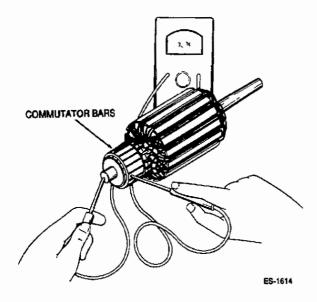
FIGURE 6-39. TESTING ARMATURE FOR GROUNDS
