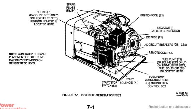
*Fuse (F2) (Spec K gensets):* This 5-amp fuse protects the fuel pump and choke heater circuit. It is mounted on the front of the control box (see Figure 7-1a).
