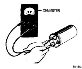
FIGURE 6-12, TESTING COIL SECONDARY
