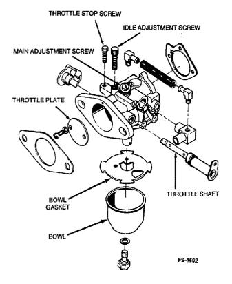
FIGURE 6-28. CARBURETOR OVERHAUL
