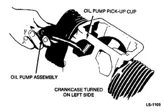
FIGURE 9-16. OIL PUMP ASSEMBLY
