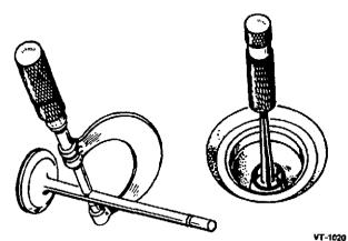
FIGURE 9-6. VALVE STEM & VALVE GUIDE INSPECTION
