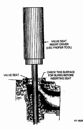
FIGURE 9-11. INSERTING NEW VALVE SEAT
