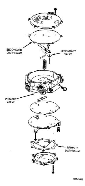
FIGURE 6-31. REGULATOR DISASSEMBLY
