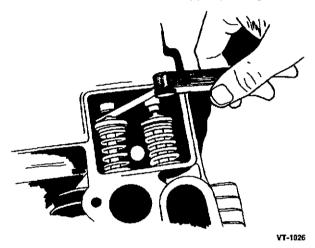
FIGURE 9-12. VALVE CLEARANCE ADJUSTMENT
