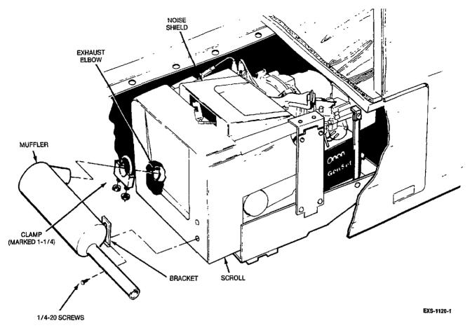
FIGURE 6-2. UNDERFLOOR MOUNT EXHAUST SYSTEM
