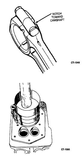
FIGURE 9-26. INSTALLING PISTON AND CONNECTING ROD
