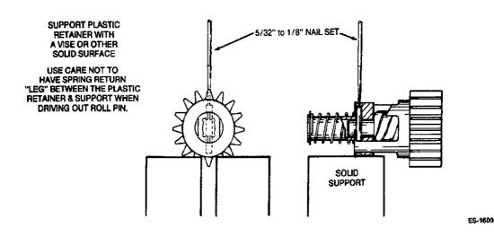
FIGURE 6-38. DRIVING ROLL PIN OUT
