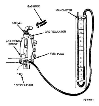
FIGURE 6-36. MANOMETER TESTING (IF REQUIRED)
