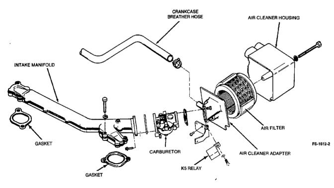
FIGURE 6-26. CARBURETOR, AIR FILTER AND INTAKE MANIFOLD ASSEMBLY
