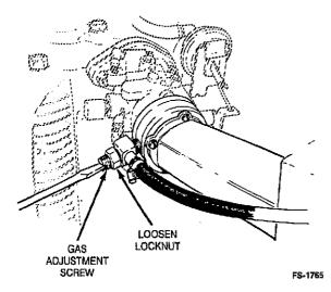
FIGURE 6-35. ADJUSTING FUEL FLOW AT CARBURETOR
