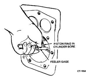
FIGURE 9-24. CHECKING RING GAP
