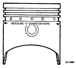
FIGURE 9-23. PISTON CLEARANCE MEASUREMENT
