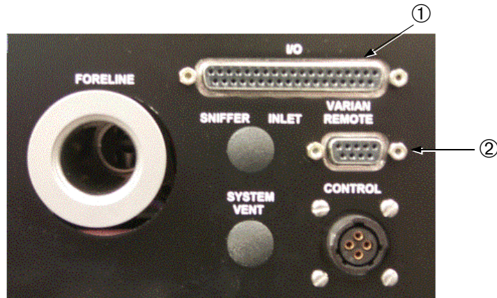
Figure A-1 System Control and Communication Panel
