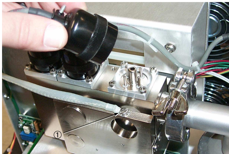
Figure 4-3 Removing the Connectors
