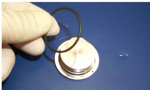
Figure 4-18 Removing the O-ring from Magnetic Pole Piece
