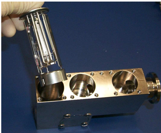
Figure 4-16 Removing the Preampifier
