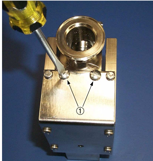
Figure 4-7 Magnet Assembly Slotted Screws
