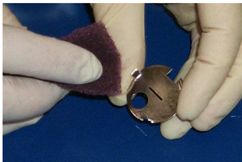
Figure 4-20 Discolored Ground Slit Plate
