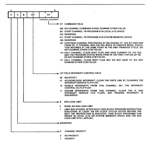
Figure 1-8. The Channel Control Word (CCW)
