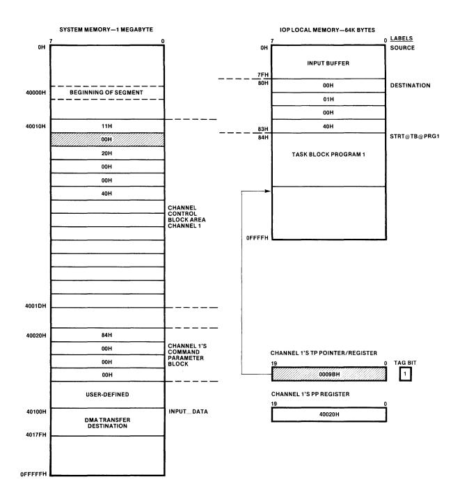
Figure 1-19. Stage Four-Task Block Program Execution Ended
