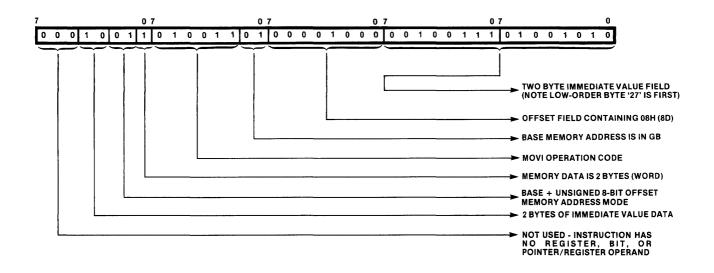
Figure 3-3. Assembled Encoding of MOVI [GB].8, 4A27H
