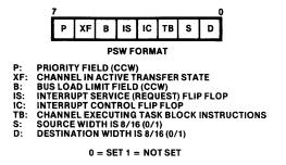
When channel operations are resumed following their suspension (101B in the Command Field of the CCW), the stored TP pointer/register and tag bit are restored from the PB by the 8089 hardware. Any changes to the PSW while it was stored will be in effect when channel operation resumes. (See figure 1-11.)
