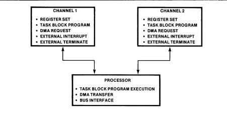
Figure 1-5. A Conceptual View of the 8089 I/O Processor
