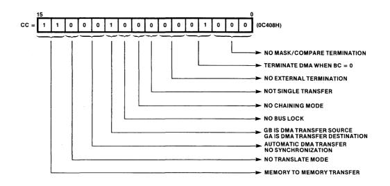
The DMA source and destination logical widths are specified by the WID 8, 8 instruction. (The IOP optimizes DMA transfers by data assembly/disassembly operations, depending on the WID instruction values and the source data address [odd or even].)
