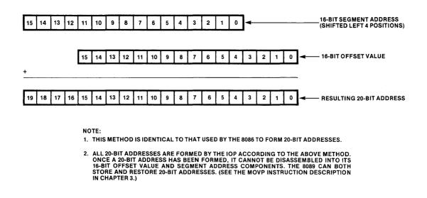
Figure 1-9. The Formation of 20-Bit Addresses by the 8089 Hardware
