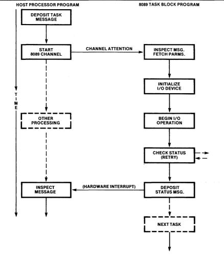
the host processor is free to do other processing. If the operation does not complete successfully, the channel takes corrective action, signalling the host processor when the I/O operation is completed or error correction routines have finished executing.
