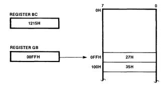
2. The instruction JBT [GA+IX], 5, ERROR\_ROUTINE tests bit five of the data memory byte located at GA + IX and jumps to the instruction labeled ERROR\_ROUTINE if the bit is true (equal to logical one).
