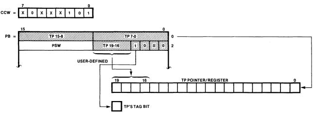
**RESUMING CHANNEL OPERATIONS FOLLOWING A CHANNEL HALT COMMAND (CCW = 110B)**
