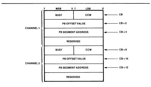
Figure 1-7. The Channel Control Block (CB)
