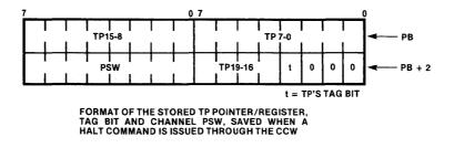
The Program Status Word (PSW) is a byte containing information on a channel's status. It is continuously updated by the 8089 but is not directly accessible by task block programs. It can only be examined when a channel's operation has been suspended, at which time it is stored in the fourth byte of the channel's PB by the 8089 hardware.
