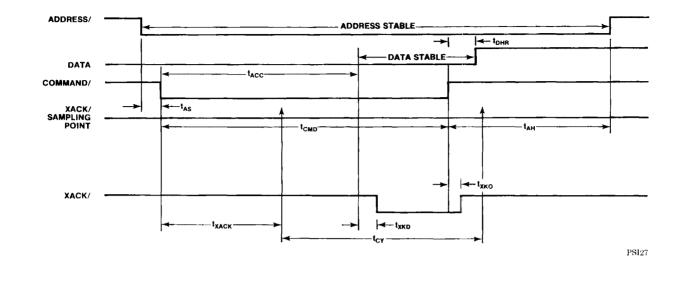
Figure 2-5. Memory and I/O Write Timing
