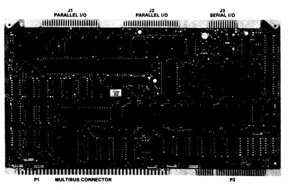
Figure 1-1. iSBC 80/10B<sup>™</sup> Single Board Computer
