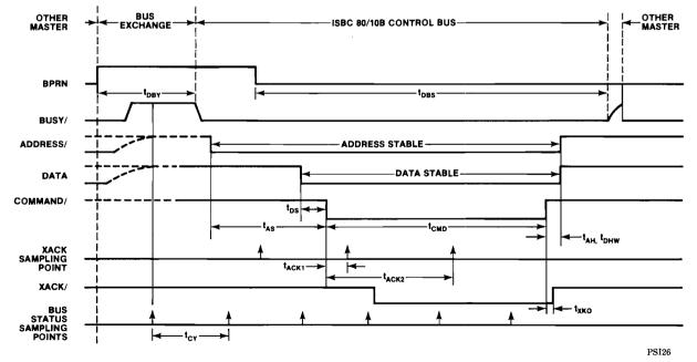
Figure 2-3. Bus Exchange Timing (Write)
