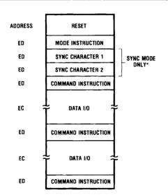
\*The second sync character is skipped if Mode instruction has programmed PCI to single character internal sync mode. Both sync characters are skipped if Mode instruction has programmed PCI to async mode.
