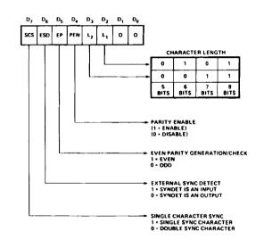
Figure 3-1. PCI Synchronous Mode Instruction Word Format
