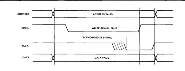
Figure 4-6. Memory and I/O Write Timing
