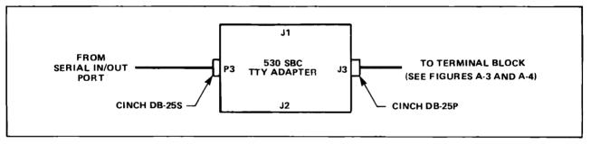
Figure B-8. TTY Adapter Cabling
