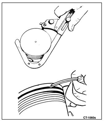
FIGURE 10-18. CLEANING RING GROOVES
