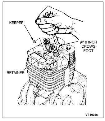
FIGURE 10-6. VALVE REMOVAL
