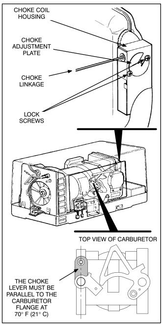
FIGURE 8-23. CHOKE ASSEMBLY (TYPICAL ALSO OF MODEL KVC)
