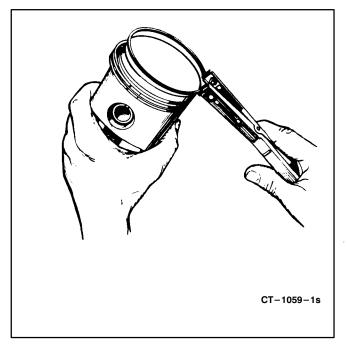
FIGURE 10-17. REMOVING PISTON RINGS
