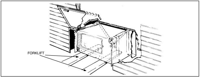
FIGURE 5-4. COMPLETE SET REMOVAL (MODEL KV)
