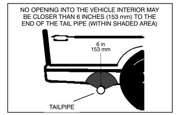
FIGURE 8-7. MINIMUM DISTANCES TO OPENINGS
