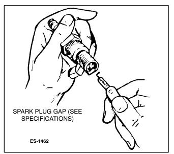
FIGURE 8-12. MEASURING PLUG GAP
