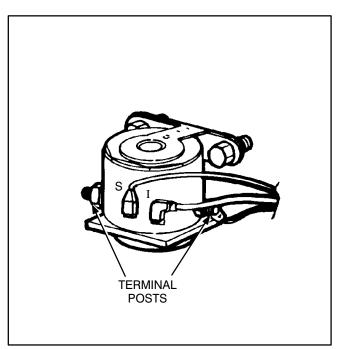
FIGURE 7-4. START RELAY CHECK
