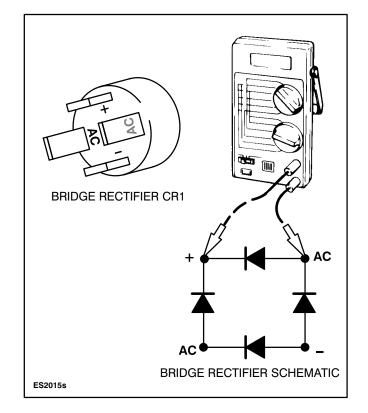
FIGURE 7-5. DIODE BRIDGE CR1 CHECK
