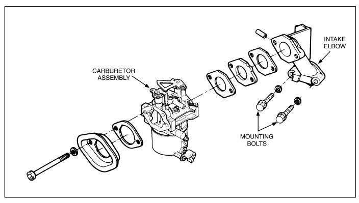
FIGURE 8-16. CARBURETOR AND INTAKE MANIFOLD ASSEMBLY
