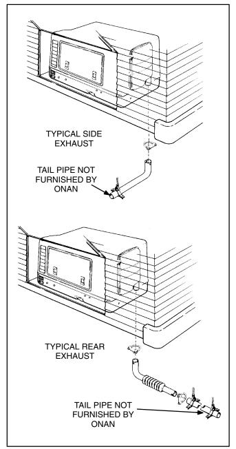
FIGURE 8-2. MODEL KV EXHAUST TAILPIPE
