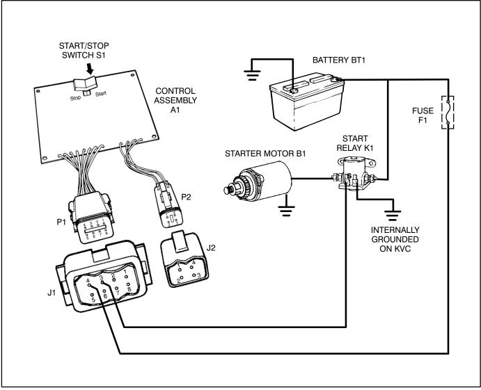
FIGURE 6-3. START – CRANKING MODE
