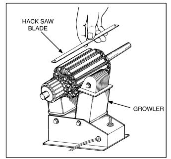
FIGURE 8-31. TESTING ARMATURE FOR SHORTS
