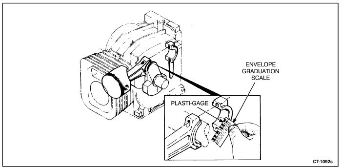
FIGURE 10-25. MEASURING CRANKPIN CLEARANCE
