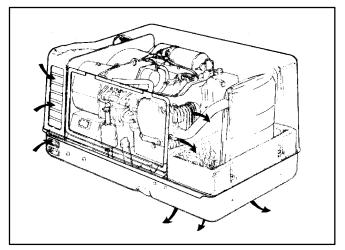
FIGURE 8-8. MODEL KV COOLING AIRFLOW
