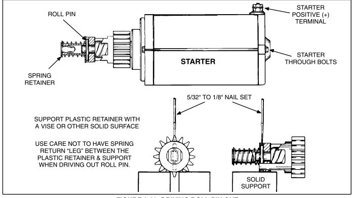
FIGURE 8-29. DRIVING ROLL PIN OUT
