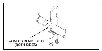
**FIGURE 8-4. TAIL PIPE CONNECTIONS**
