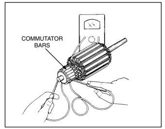
FIGURE 8-30. TESTING ARMATURE FOR GROUNDS
