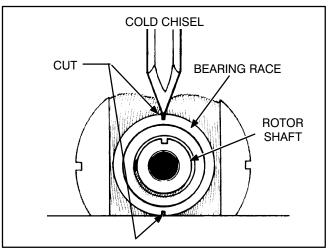
FIGURE 9-12. ROTOR BEARING REMOVAL
