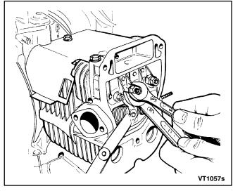
FIGURE 10-12. VALVE LASH ADJUSTMENT
