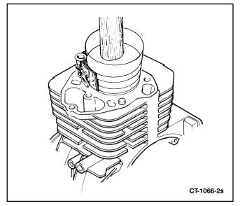
FIGURE 10-24. INSTALLING PISTON
