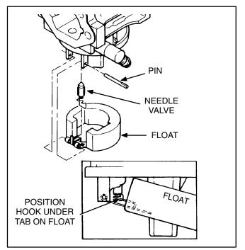
FIGURE 8-21. FLOAT INSTALLATION (PRIOR TO SPEC E, MODEL KV ONLY)
