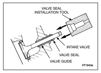
FIGURE 10-11. VALVE SEAL INSTALLATION
