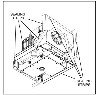
FIGURE 8-11. AIR SEALING STRIPS (MODEL KVC)
