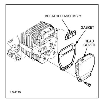
FIGURE 10-3. HEAD COVER REMOVAL
