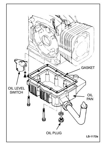
FIGURE 10-2. OIL PAN REMOVAL
