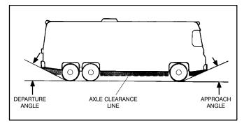
FIGURE 8-5. APPROACH AND DEPARTURE ANGLES AND AXLE CLEARANCE
