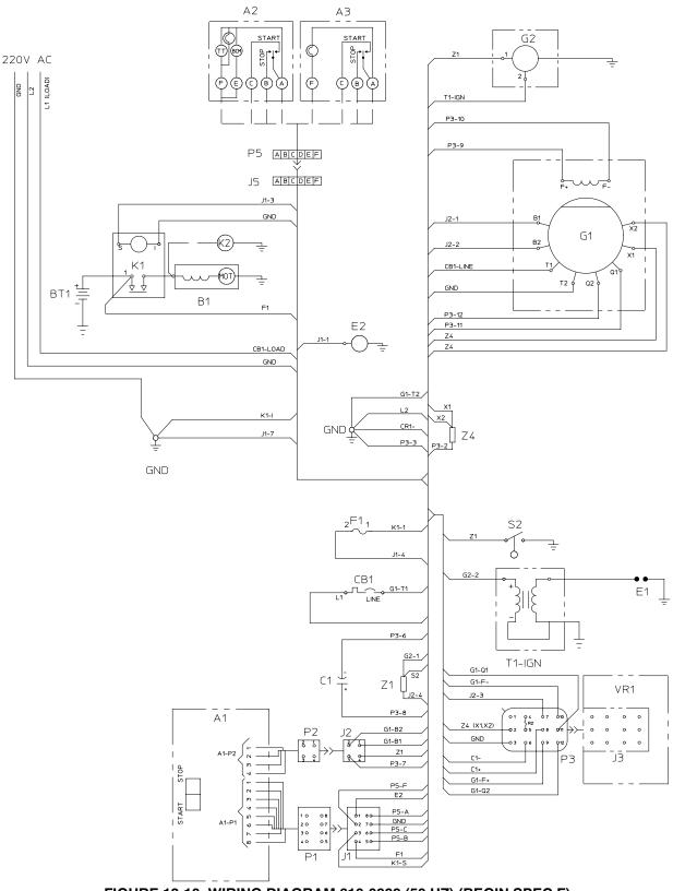
FIGURE 12-10. WIRING DIAGRAM 610-0389 (50 HZ) (BEGIN SPEC F)
