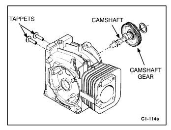
FIGURE 10-14. CAMSHAFT AND TAPPETS
