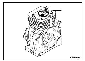
FIGURE 10-16. REMOVING WEAR RIDGE
