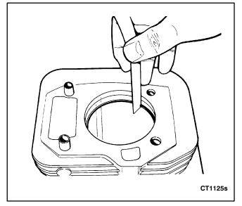
FIGURE 10-22. CHECKING RING GAP
