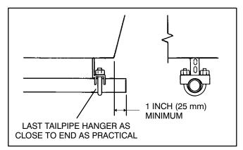
FIGURE 8-6. TERMINATING THE TAIL PIPE
