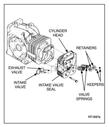
FIGURE 10-5. OVERHEAD VALVE SYSTEM
