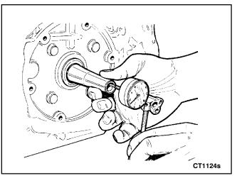
FIGURE 10-26. CHECKING ENDPLAY
