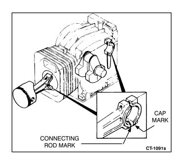
FIGURE 10-23. ROD CAP ASSEMBLY
