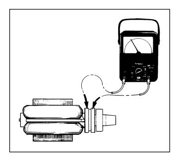
FIGURE 9-5. OPEN OR SHORTED ROTOR TEST
