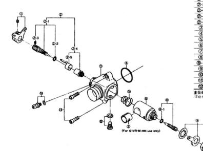
carburettor periodically. Using the wrench supplied, remove the needle-valve holder from the carburettor body and wash out the interior to remove any minute particles that may have escaped through the filters.
