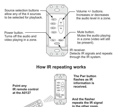
Be sure the flasher is attached directly over the component's IR receiver.
