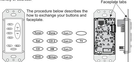
1 Detach the existing faceplate by pressing the plastic tabs with a flat blade screwdriver. (Press inward and upward () at a 30 degree angle)
