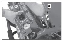
Connect air hose (sold separately) to quick connect plug (b) and quick connect (a). The console can then be brought closer to the work site to rest on the console brackets (d) or be temporarily mounted using the mounting hole (c).
