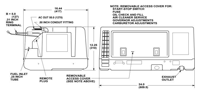
Dimensions in parentheses are millimeters. This outline drawing is provided for general reference only and is not intended for design or installation. For more information see installation manual or obtain outline drawing 500-2182 and wiring diagram from your Distributor/Dealer.
