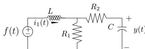
where  $R_1 = 1 \text{ k}\Omega$ ,  $R_2 = 22 \text{ k}\Omega$ ,  $C = 10 \mu\text{F}$ , and  $L = 5 \text{ H}$ .
