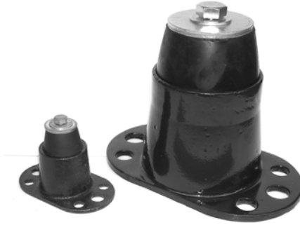
Figure 5-3 Seismically rated elastomeric mounts. The mount on the left (75 mm tall) has a nominal load rating of about 40 kg. The mount on the right (165 mm tall) has a nominal load rating of as much as 700 kg.
