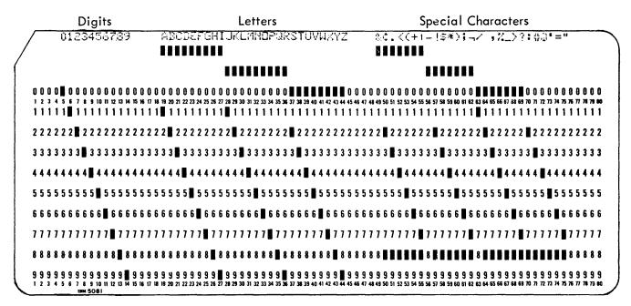
Figure 9. Standard IBM System/360 Card Code
