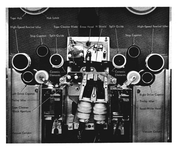
Figure 8. IBM 2401-2404 Transport, Models 2, 3, 5, or 6
