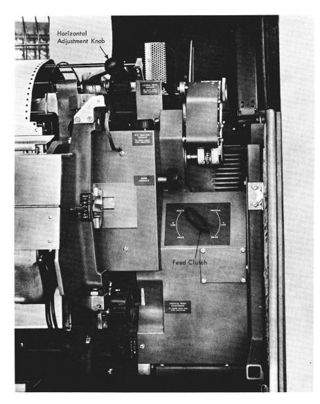
Figure 13. Carriage Controls
