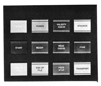
Figure 10. Reader Controls and Common Indicator Lights
