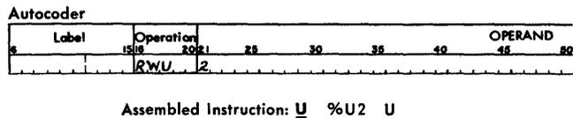
Figure E-14. Rewind Tape and Unload
