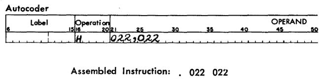
Figure B-40. Coded Halt
