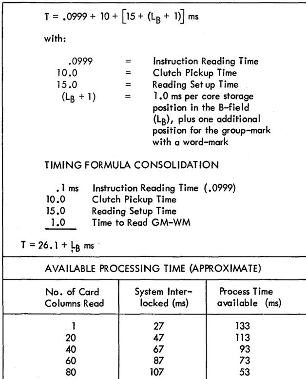
Figure D-38. IBM 1442, Model 2; Timing—375 cpm
