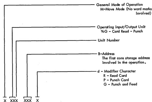
Figure D-24. IBM 1442 Card Read-Punch Instruction Format
