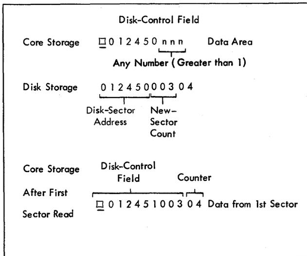
Figure F-6. Read Disk - Sector-Count Overlay Operation
