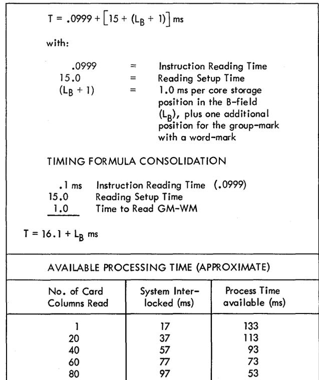
Figure D-40. IBM 1442, Model 2; Timing—400 cpm
