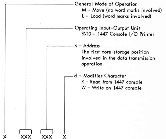
Figure C-2. IBM 1447 Console I/O Printer Instruction Format
