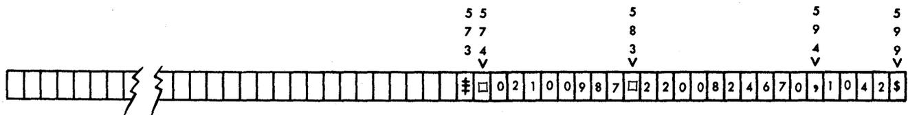
Figure G-29. Data Read into Storage, First Amount Symbol Not Identified
