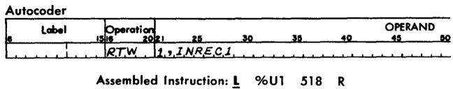
Figure E-5. Read Tape with Word Marks (Load Operation)
