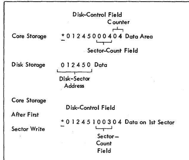
Figure F-31. Write Disk - Sector-Count Overlay Operation
