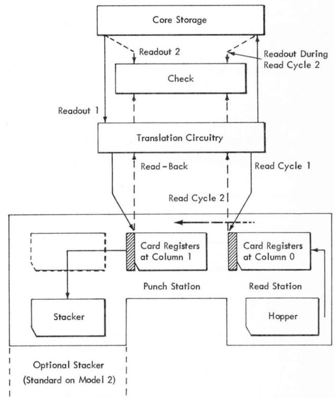
Figure D-23. IBM 1442 Card Read-Punch Data Flow
