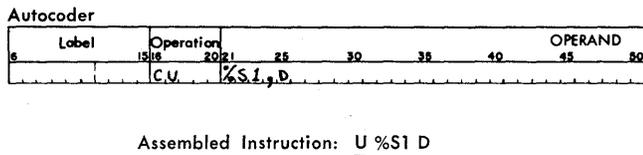
Figure G-15. Disengage Magnetic Character Reader
