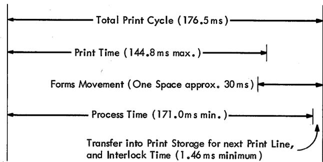
Figure D-5. Print Operation Timing Chart—
