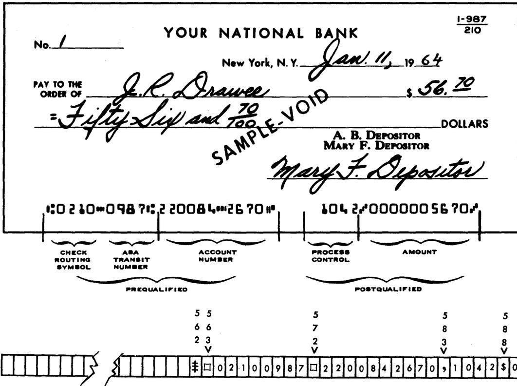
Figure G-28. Inscribed 6-Inch Check Read into Storage Correctly
