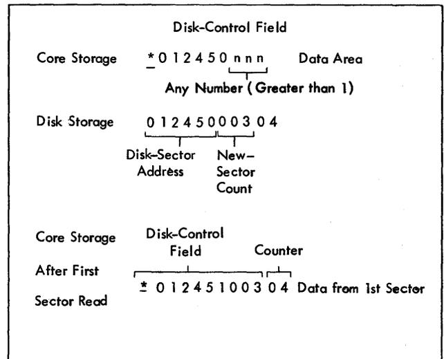
Figure F-27. Read Disk - Sector-Count Overlay Operation
