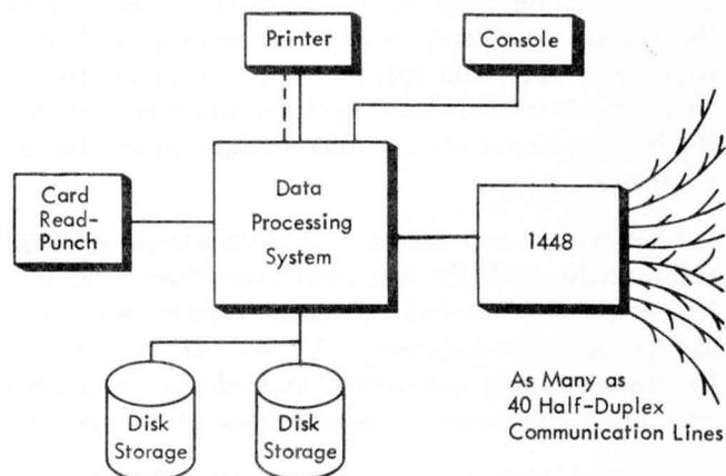
Figure G-32. The Processor Controls as Many as 40 Half-Duplex Channels
