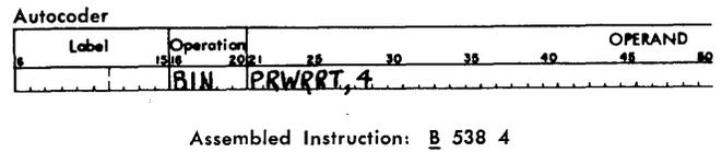
Figure H-35. Branch If Primary-Write Indicator On
