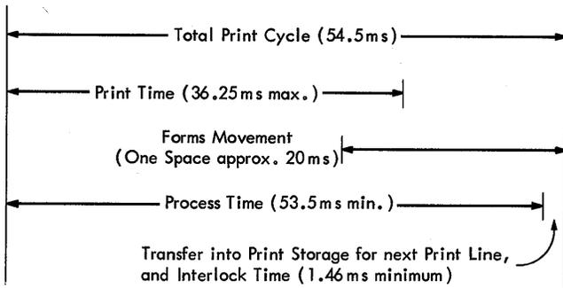
Figure D-3. Print Operation Timing Chart—
