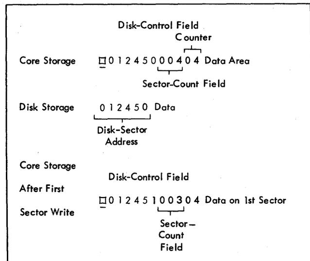
Figure F-10. Write Disk - Sector-Count Overlay Operation
