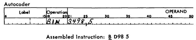
Figure G-10. Branch If End-of-Message Receive Indicator On
