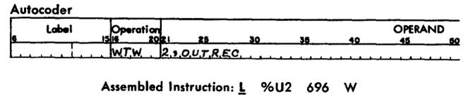
Figure E-8. Write Tape with Word Marks
