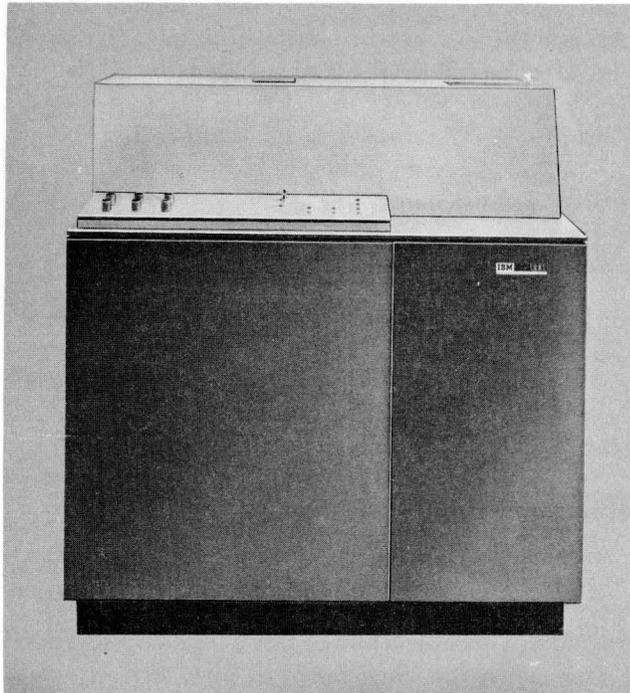
Figure G-51. IBM 1231 Optical Mark Page Reader
