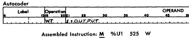
Figure E-6. Write Tape (Move Operation)
