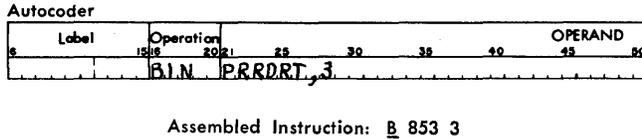
Figure H-34. Branch If Primary-Read Indicator On
