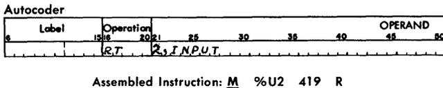
Figure E-3. Read Tape (Move Operation)
