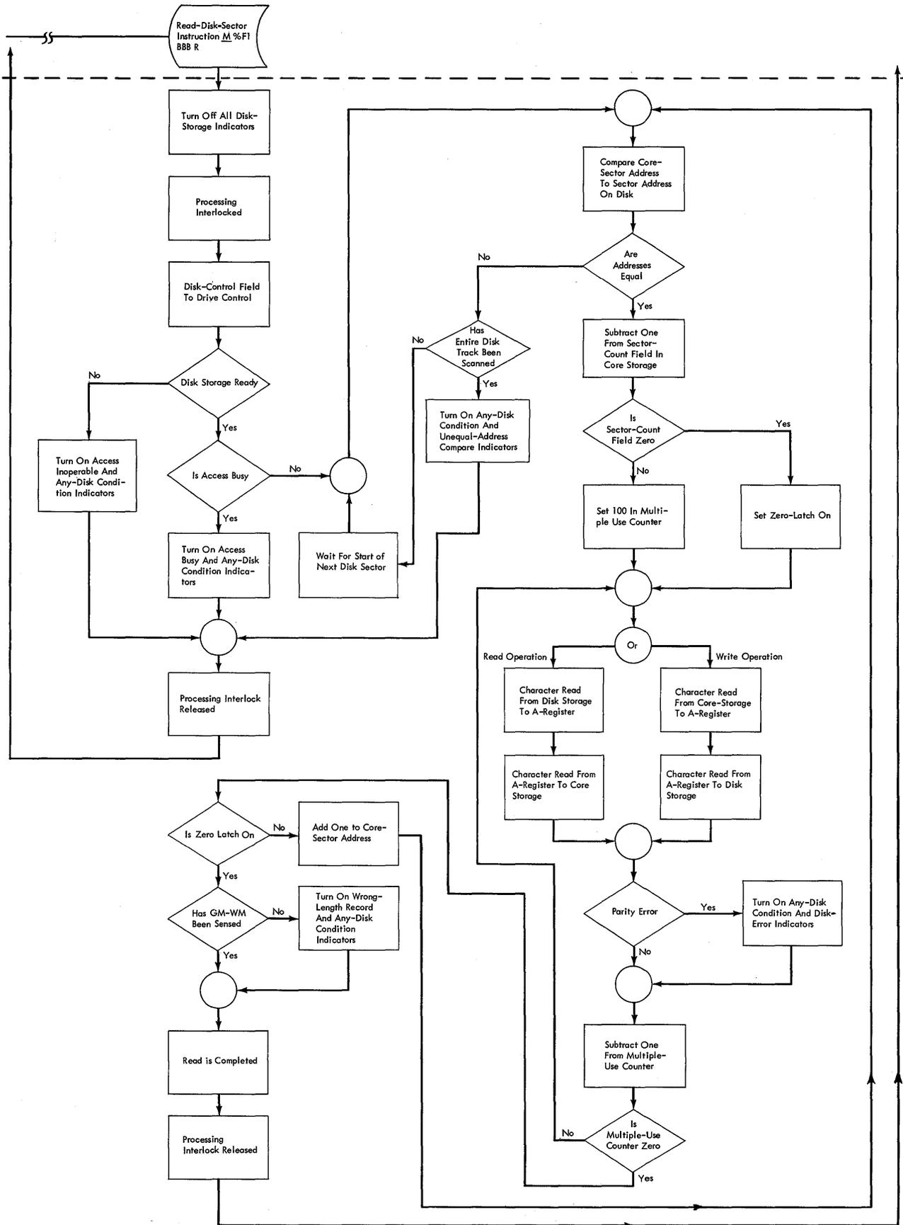
Figure F-24. Read/Write Disk Functional Schematic
