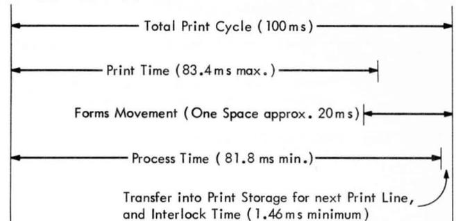
Figure D-2. Print Operation Timing Chart—
