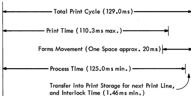
Figure D-4. Print Operation Timing Chart—
