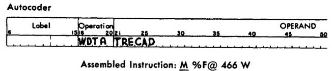
Figure H-72. Write Disk-Track Record with Address
