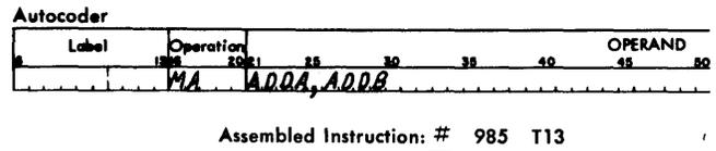
Figure A-15. Modify Address (Two Addresses)
