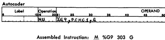
Figure H-87. Punch-and-Feed in Card Image Mode
