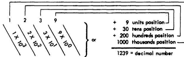
As shown above, the decimal number system allows counting to ten in each position—from units to tens to hundreds to thousands etc. The binary system allows counting to two in each position. Register displays in the System/360 are in binary form: a bit light on is a "one" a bit light off is a "zero".
