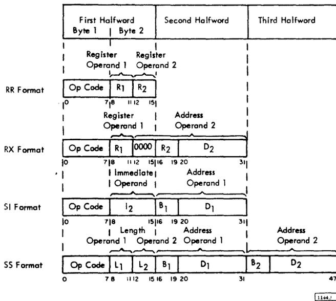
In each format, the first instruction halfword consists of two parts. The first byte contains the operation code (op code). The length and format of an instruction are specified by the first two bits of the operation code. The second byte may be used to contain data, specify operand lengths, or specify registers to be used by the operation.
