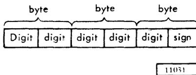
The decimal digits range from 0 to 9 while any value from 10 to 15 (in hexadecimal representation 'A' to 'F') is regarded as a valid sign. In decimal arithmetic, all numbers must be arranged in the packed format. By means of the Pack instruction,
