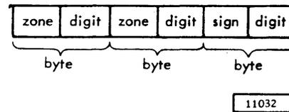
The left four bits of each byte in this format are called zone bits, and are not used except for the low-order (rightmost) byte which uses them for the sign. Zone bits do not affect the value of the numeric digit contained in the right four bits of the byte.
