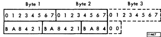
check is set to indicate that zeros must be subtracted to obtain the original character bit configuration. The same holds true for one tape character because it also does not fill one byte completely. One tape character is transmitted as one byte with the bits 6 and 7 of that byte set to zero and the data converter check turned on.
