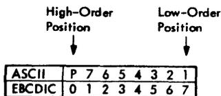
Figure 12. Sequential Numbering of Bit Positions in ASCII and EBCDIC
