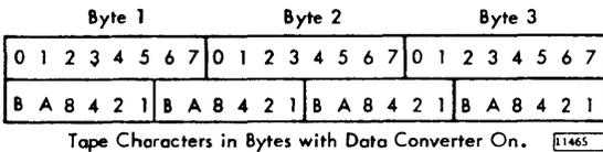
Whenever less than four characters are transferred, a special packing arrangement is employed. For example, two tape characters are packed into one byte if the character bits 8, 4, 2, 1 are all zeros. However, when the bits 8, 4, 2, 1 are not all zero, the two characters are set into two bytes with the bits 4, 5, 6, 7 of the second byte set to zero and the data converter check turned on.
