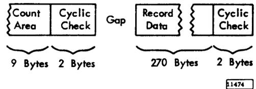
As data is transferred from the CPU to an attached storage device, the storage control computes two cyclic check bytes which are added to the end of each area. The two cyclic check bytes are arithmetically coded to represent the data in the associated area.
