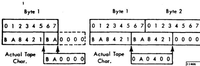
When successfully packed characters are read back, zeros must be added to retrieve the original character. The data converter check indicates that zeros must be subtracted to obtain the original character. Three tape characters are packed into two bytes if bits 2 and 1 of the third character are zero; if they are not, a third byte is used with the bits 2, 3, 4, 5, 6, and 7 set to zero. The data conversion
