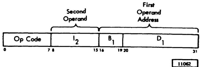
In the SI format, the address which specifies the core storage location of the first operand field is derived from the contents of the B1-D1 fields of the instruction. The address may be taken directly from the B1-D1 Fields (direct addressing) or an effective address may be formed by adding the contents of the general register specified by the B1 field to the contents of the D1 field (effective addressing).
