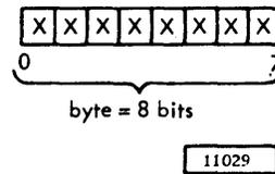
Main storage is used to hold all the data that is to be operated upon, or processed, at a given time. It also holds the instructions, or program, which control the operation of the system. For each individual job performed by the system, certain portions
