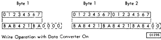
If a 7-track tape was written on another system (for example, IBM 1401 Processing Unit), reading is as follows.
