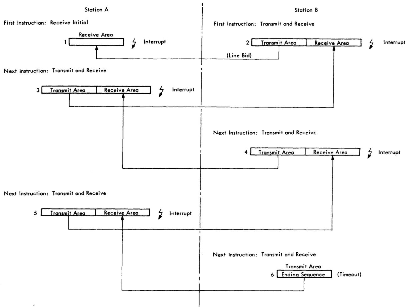
Figure 16. Data Exchange via Transmit and Receive
