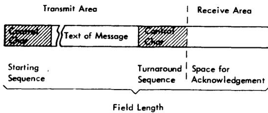
Figure 13. Transmit and Receive Instruction used by Donor 01264
