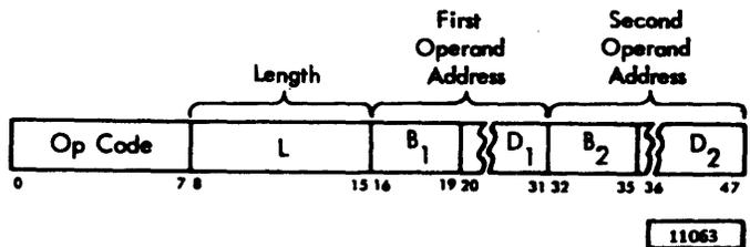
The address which specifies the core-storage location of the first operand field is derived from the B1-D1 fields of the instruction. The B2-D2 fields specify the leftmost byte of the second operand field. The first and second operand fields are the same length. The number of bytes extending to the right of the first byte is specified by the L field of the instruction.
