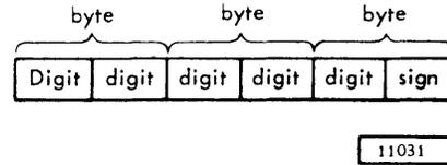
An eight-bit byte may contain two numeric digits, except in the case of the rightmost byte, which has a sign to the right. Variable field length in this format allows for fields up to 16 bytes in length.
