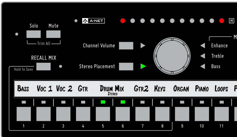
Channel 5-6 are stereo linked at a Pro16 input device when in 16-channel mode.
