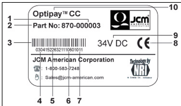
Figure 3-4 Coin Validator Side Label
