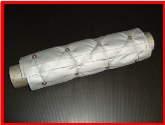
Removable blanket sections are assembled with either locking wire or spring clips with hook fasteners mounted on the fabrics.
