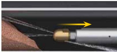
LE SYSTÈME AUTOSTROKE "DÉTECTE" L'OBSTRUCTION ET RAMÈNE LÉGÈREMENT LE FLEXIBLE EN ARRIÈRE POUR RÉCUPÉRER LA ROTATION DE LA TÊTE.
