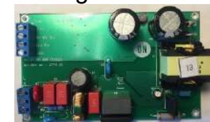
20 W 0-10, PWM Dimming Driver
