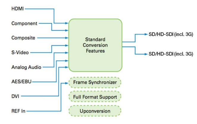
HDMI & SDI to Analog & SDI Multi-Functional Converter/Scalar with Frame Synchronizer
