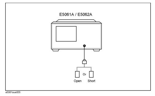
Step 7. Press Open or Short to start the calibration measurement.
