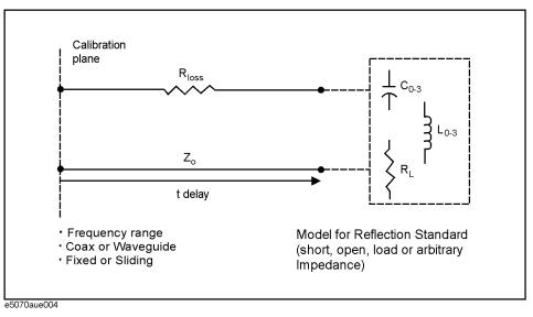
Figure 4-21 Transmission Standard Model (THRU)
