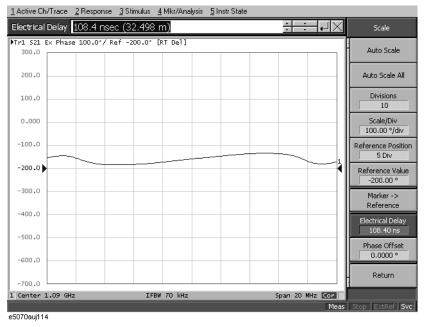
**Measurement Examples** Measuring the Deviation from a Linear Phase
