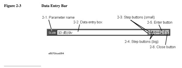
NOTETo manipulate the data entry bar using the front panel keys, the data entry bar must be<br/>selected as the object to be manipulated (with the focus placed on it). When the focus is<br/>placed on the data entry bar, the entire bar is displayed in blue. Pressing or clicking <a href="#">Focus</a><br/>in the "8. ENTRY Block" on page 28 enables you to move the focus to the desired object.
