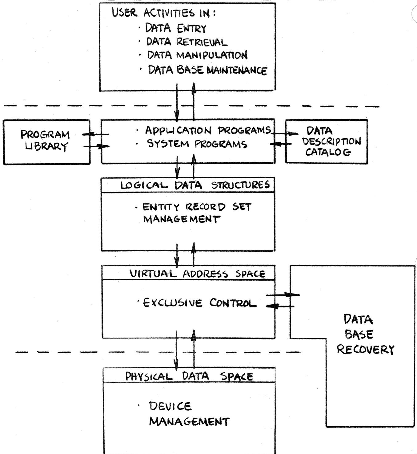
FIGURE 3.4.1.1-1: A LOGICAL REPRESENTATION OF DATA BASE COMPONENTS & INTERFACES
