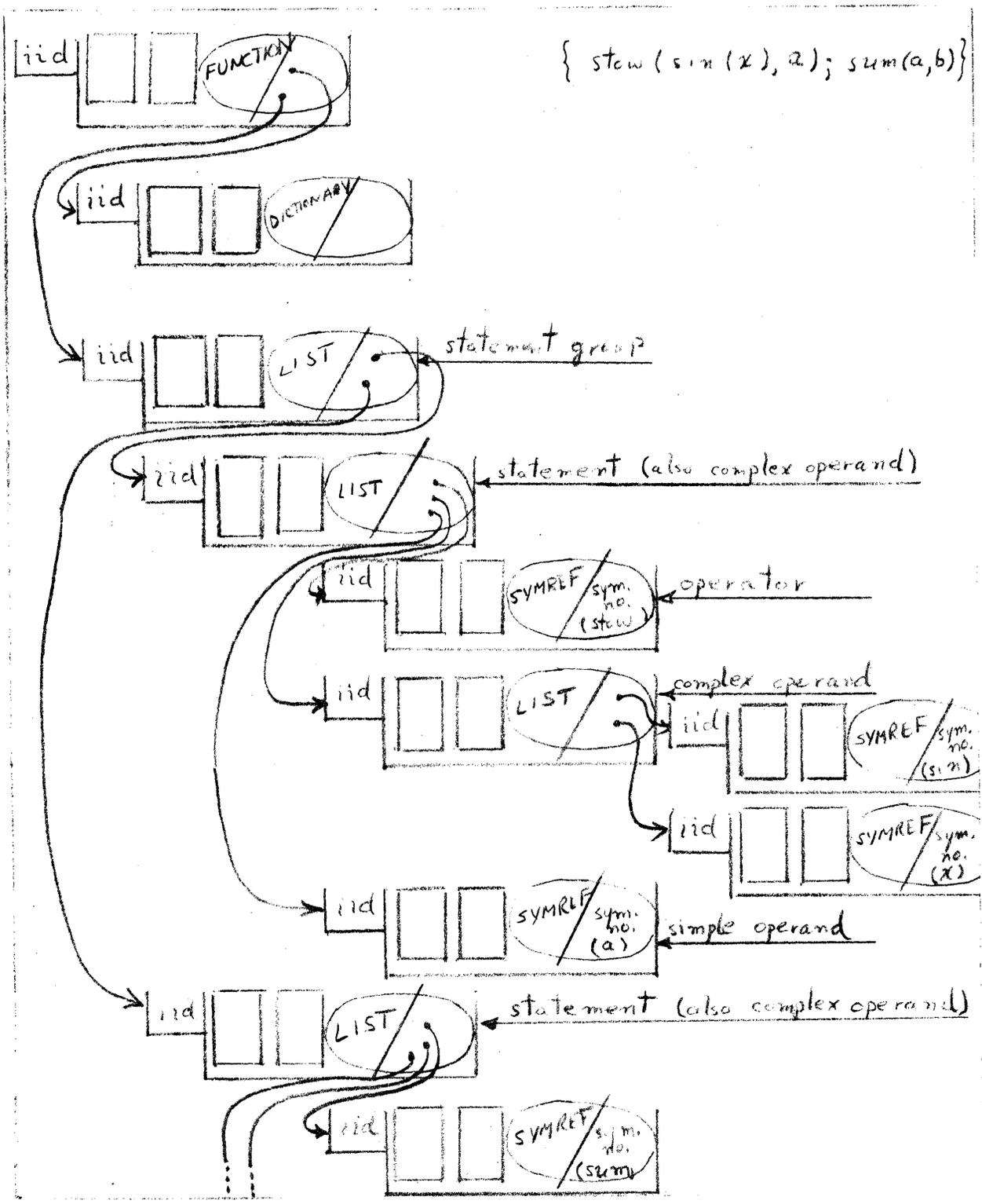
Figure 5.3.2-1: Structure of a Sample Function
