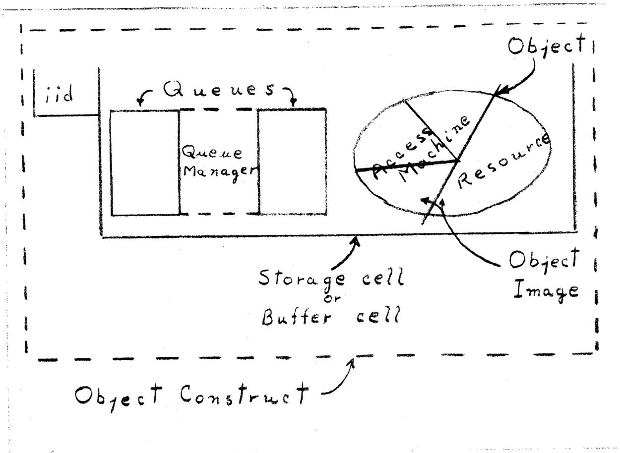
Figure 5.1-1: Structure of a Storage Cell and its Contents
