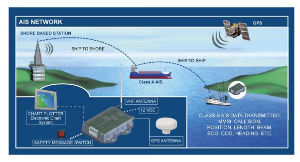
On the bottom, a typical Nauticast™-B AIS installation in a common environment is shown. The Nauticast™-B AIS is connected to the vessel's power supply, and, in connection with the VHF and GPS antennas, the minimal requirements for transponder operation are fulfilled.
