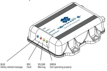
If the red LED illuminates continuously, the unit should be assumed to be faulty. It should either be switched off (power removed) or, if this is not practical, any other vessel position information derived from the unit should not be used. It should also be assumed that the unit is not transmitting valid position information for your vessel.
