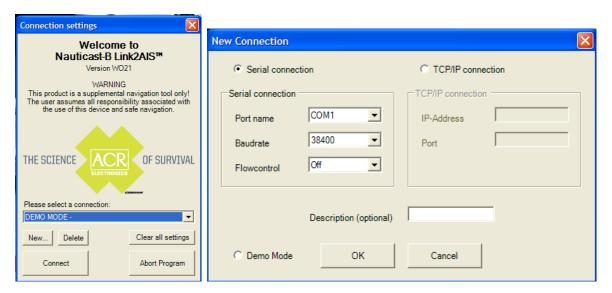
The application requires a serial connection to a Nauticast™-B AIS transponder. Connect the transponder to an available serial port. If your serial port is not located in the drop down box, select 'New...' and create a new connection.
