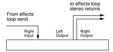
**Application** Patching into a guitar amp with a mono send and stereo return effects loop. Do not confuse this with the QuadraVerb GT's internal effects loop; the loop in an amplifier is specifically designed for the insertion of signal processors such as the QuadraVerb GT.
