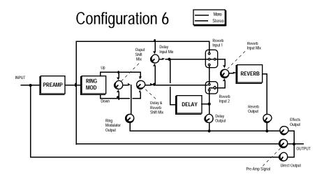
This configuration features the Ring Modulation in conjunction with Delay and Reverb. The Ring Modulator is not available in other configurations.
