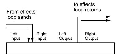
**Application** Patching into a guitar amp with a stereo send and stereo return effects loop. Do not confuse this with the QuadraVerb GT's internal effects loop; the loop in an amplifier is specifically designed for the insertion of signal processors such as the QuadraVerb GT.
