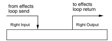
**Application** Patching into a guitar amp with a mono effects loop. Do not confuse this with the QuadraVerb GT's internal effects loop; the loop in an amplifier is specifically designed for the insertion of signal processors such as the QuadraVerb GT.
