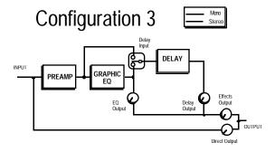
This combines the 11 band graphic EQ with delay. The EQ provides sophisticated sound-shaping for the preamp sound, and the delay adds ambience for lead effects.
