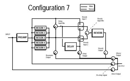
This configuration features the Resonators in conjunction with Delay and Reverb.
