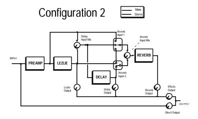
This is similar to the QuadMode™ configuration, but replaces the EQ and Pitch modules with a Lezlie (rotating speaker simulator) module and does not have a Preamp level control.
