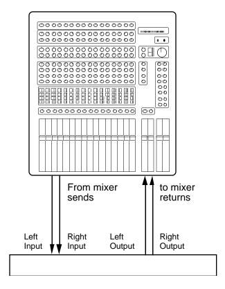
**Application** Patching into a mixer's stereo effects sends for use as a reverb or other processor while recording.
