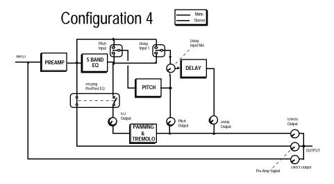
This is just the ticket for rich chorus sounds. Use the 5 Band EQ to shape your timbre, Pitch Change to add chorusing (or other pitch effects such as flanging, etc.), and Delay to add evocative echo effects. Using the Multi Tap option in the Delay module creates unusual echo effects along with chorusing.
