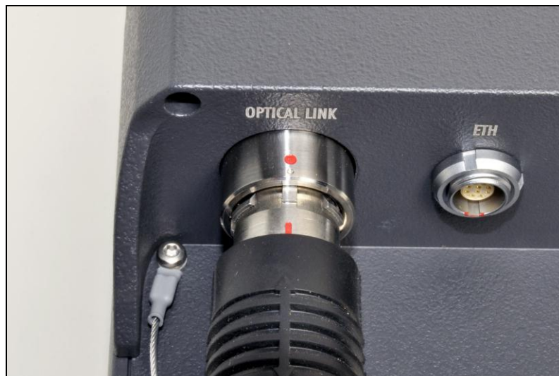
Figure 100: Correctly aligned fibre connectors
